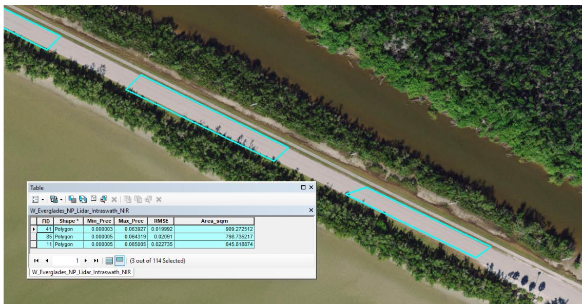
Figure 7. Intraswath polygons used to test intraswath vertical accuracy
