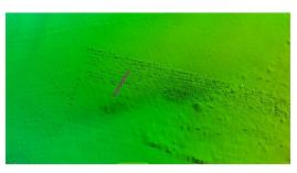
**Digital Elevation Model (DEM)** – a DEM is a digital representation of the earth's surface. See also *Digital Surface Model* and *Digital Terrain Model*.
