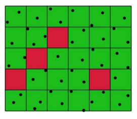
within that grid cell as indicated in the graphic at right. If at least one return falls within a cell then that cell is counted as a populated cell. If not, that cell is counted as one void of returns. If hydro breaklines were collected for the project then any cell that either touches a hydro breakline, or falls entirely within a hydro breakline is removed from the test.
