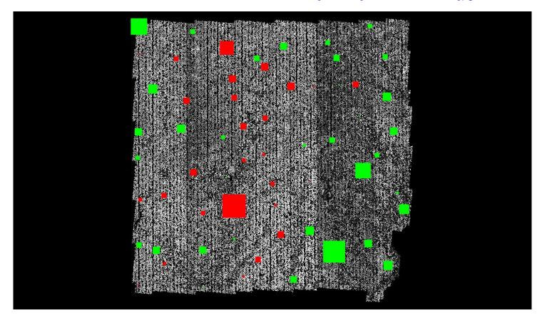
Green represents where a DEM of the lidar surface is above the check point (positive elevation error).
