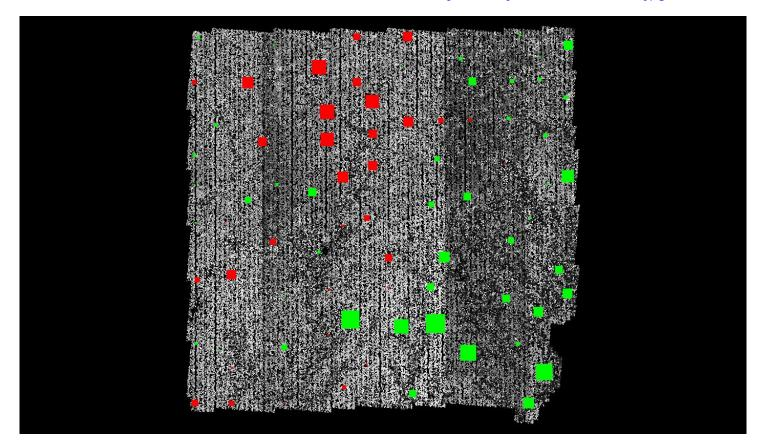
Green represents where the lidar surface is above the check point (positive elevation error).
