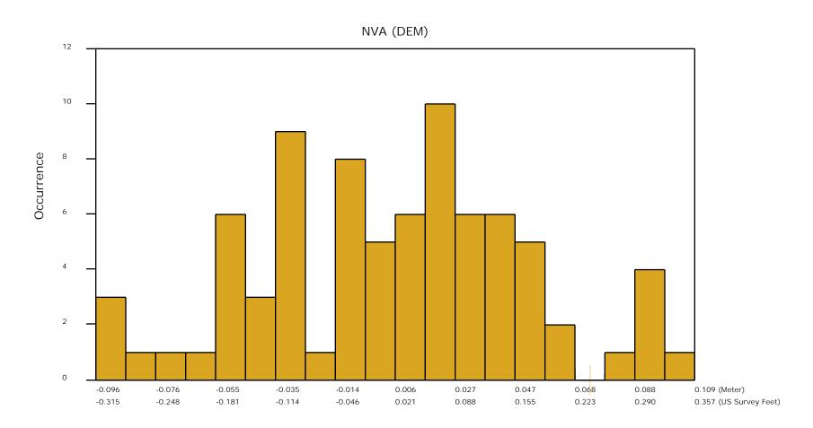
The purpose of this section is to show a frequency distribution chart of the vegetated vertical accuracy (VVA) of the DEM data measured against surveyed ground check points.
