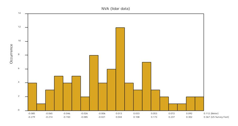
The purpose of this section is to show a frequency distribution chart of the vegetated vertical accuracy (VVA) of the lidar point cloud data measured against surveyed ground check points.
