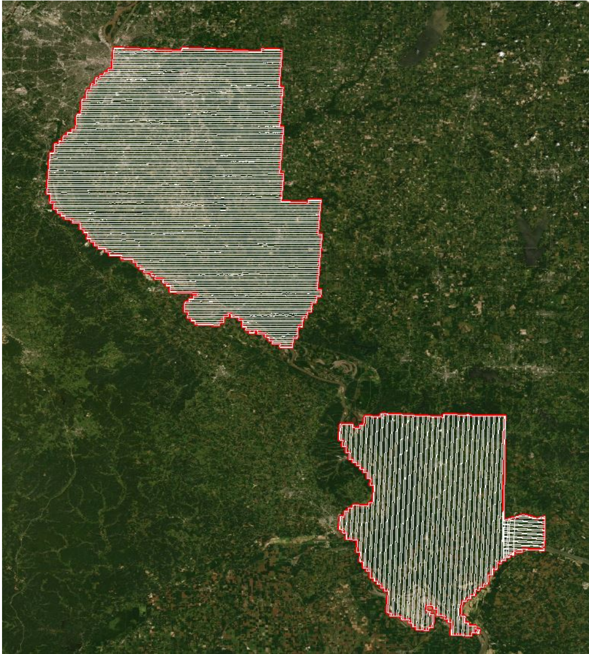
Figure 6: LiDAR swath output showing complete coverage
