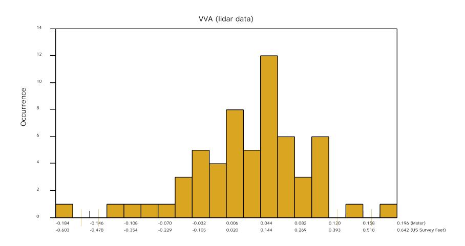
The purpose of this section is to show a frequency distribution chart of the non-vegetated vertical accuracy (NVA) of the DEM data measured against surveyed ground check points.
