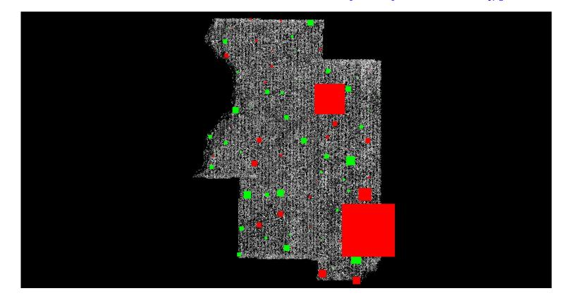
Green represents where the lidar surface is above the check point (positive elevation error).
