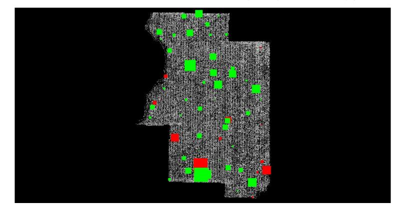
Green represents where a DEM of the lidar surface is above the check point (positive elevation error).
