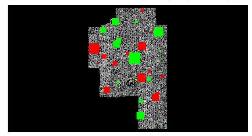
Green represents where a DEM of the lidar surface is above the check point (positive elevation error).
