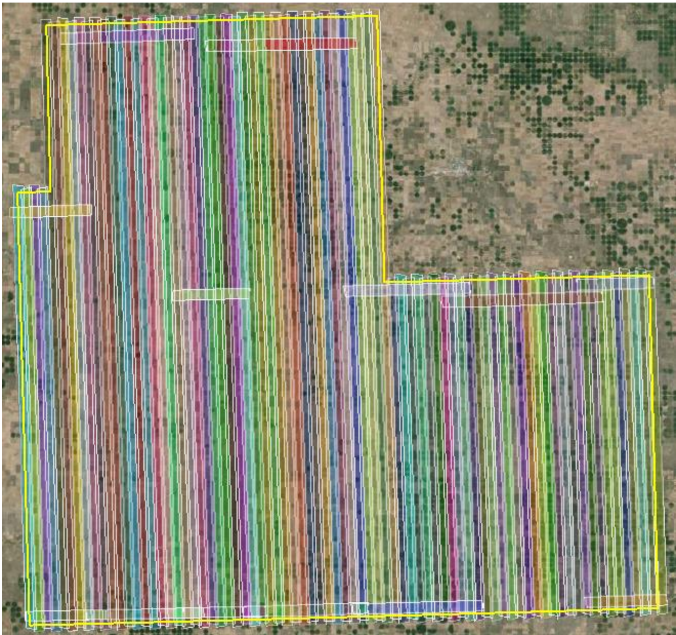
Figure 3: Lidar swath data showing complete coverage
