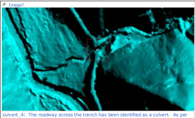
ulvert\_4: The roadway across the trench has been identified as a culvert. As per USGS Lidar Base Specification Version 1.0, roadways over culverts should not be removed from the DEM. In some instances, the roadway has been partially removed above some culverts; these roadways should be completely restored. A total of 16 culverts have been identified as errors, whereas the roadway should be restored in the DEM. (7/8/2013)
