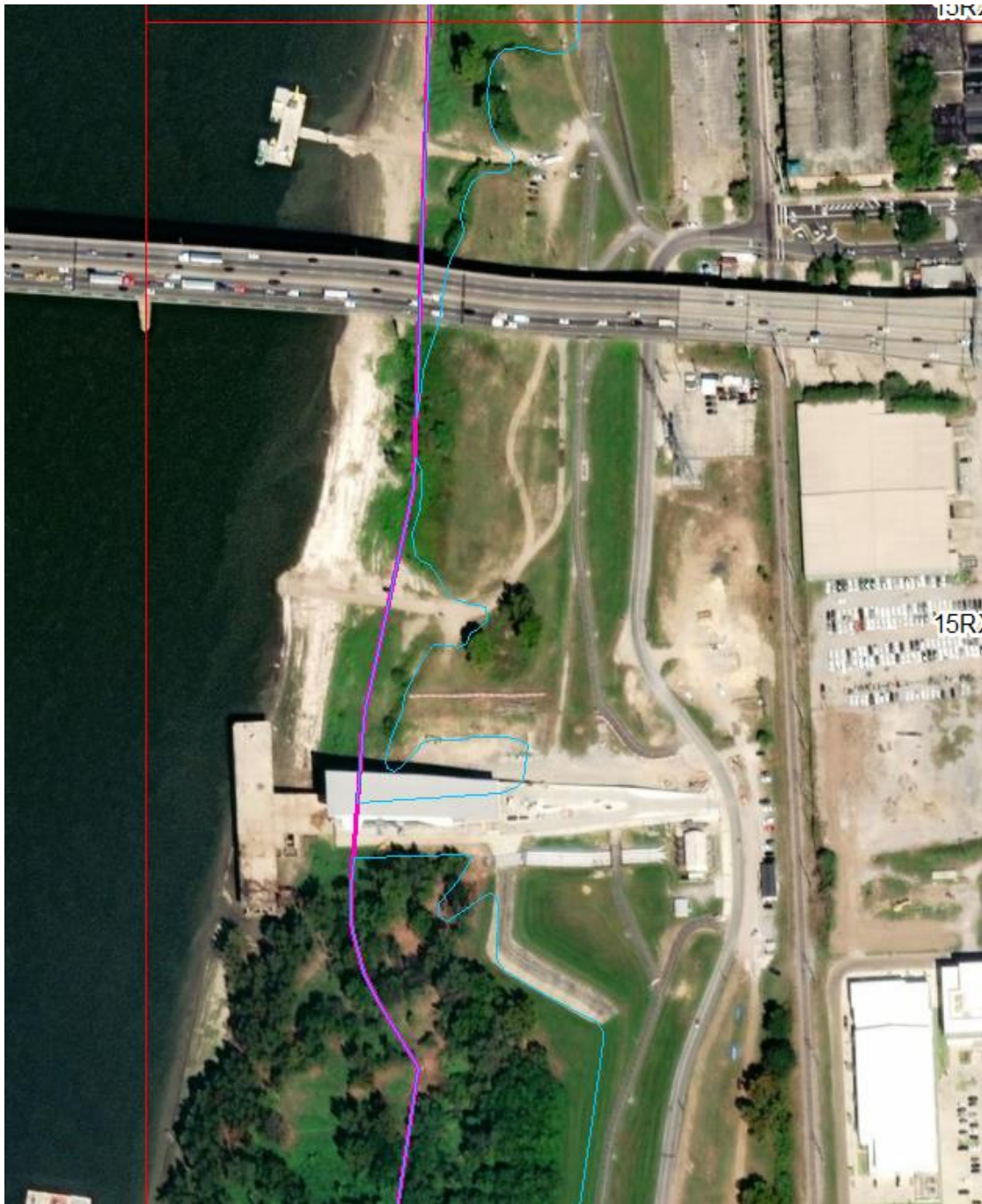
Figure 24 - Tile number 15RXP7367. The DEM image on top shows what looks to be artifacts in the water, however in the intensity image and basemap imagery on the bottom, a pier can easily be seen above the water (shown in blue, with the project buffered boundary shown in pink). Given that the water elevation was so high at the time of acquisition, the water is nearly covering the pier. Since the water is abnormally high here, the decision was made to leave the remaining ground points in the data, making it appear as if there are artifacts in the water.
