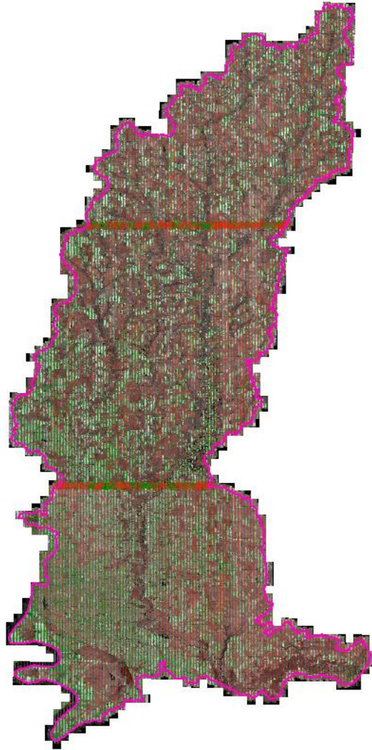
Figure 7– Single return DZ Orthos for the LA DOTD Amite Watershed Lidar Project. Inter-swath relative accuracy passes specifications. Due to the very dense vegetation in this project, many areas of the DZ Orthos show failing in red, however this data passes inter-swath accuracy in the flat open areas.
