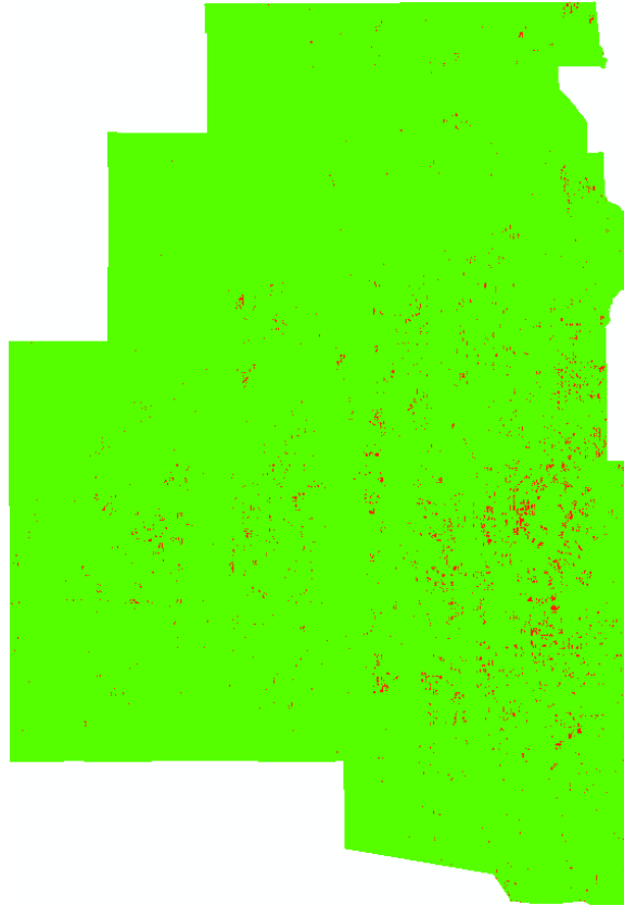
Figure 7. Density raster generated from first-return lidar pulses to ANPD of the lidar data. Green pixels are areas with 8 ppsm or greater. Red pixels contain less than 8 ppsm. The red areas are attributed to the abundance of aquaculture ponds in the center of the project area.
