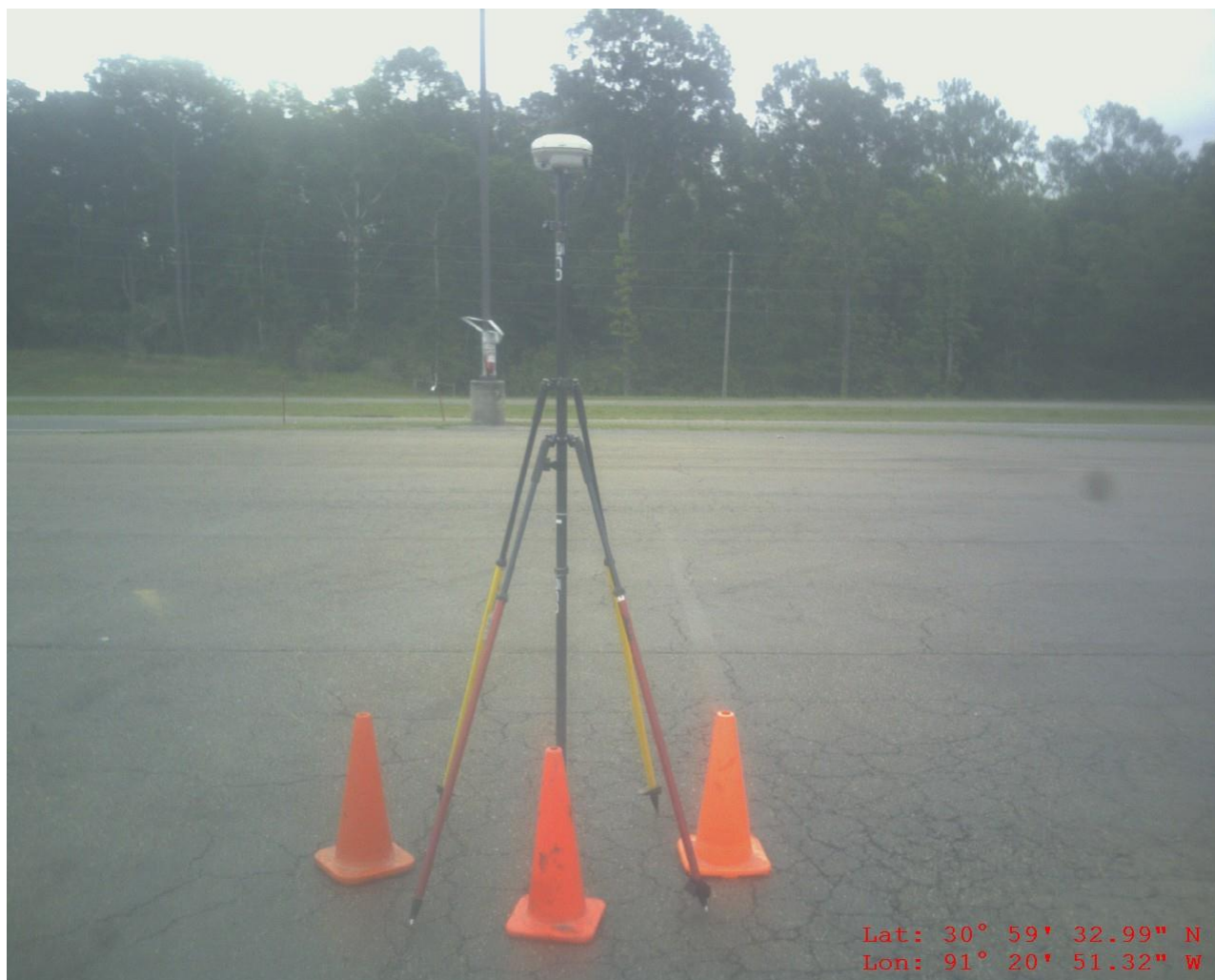
AOI-2 GCP 004 Asphalt road
