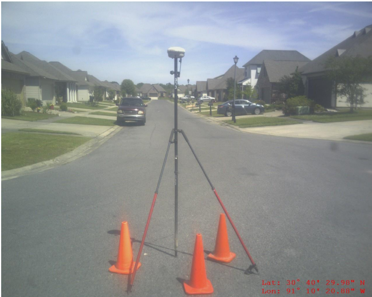
AOI-2 GCP 008 Asphalt road
