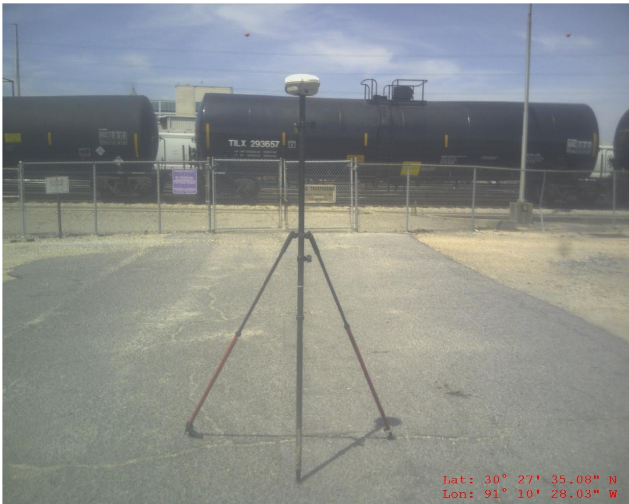
AOI-2 GCP 012 Asphalt road
