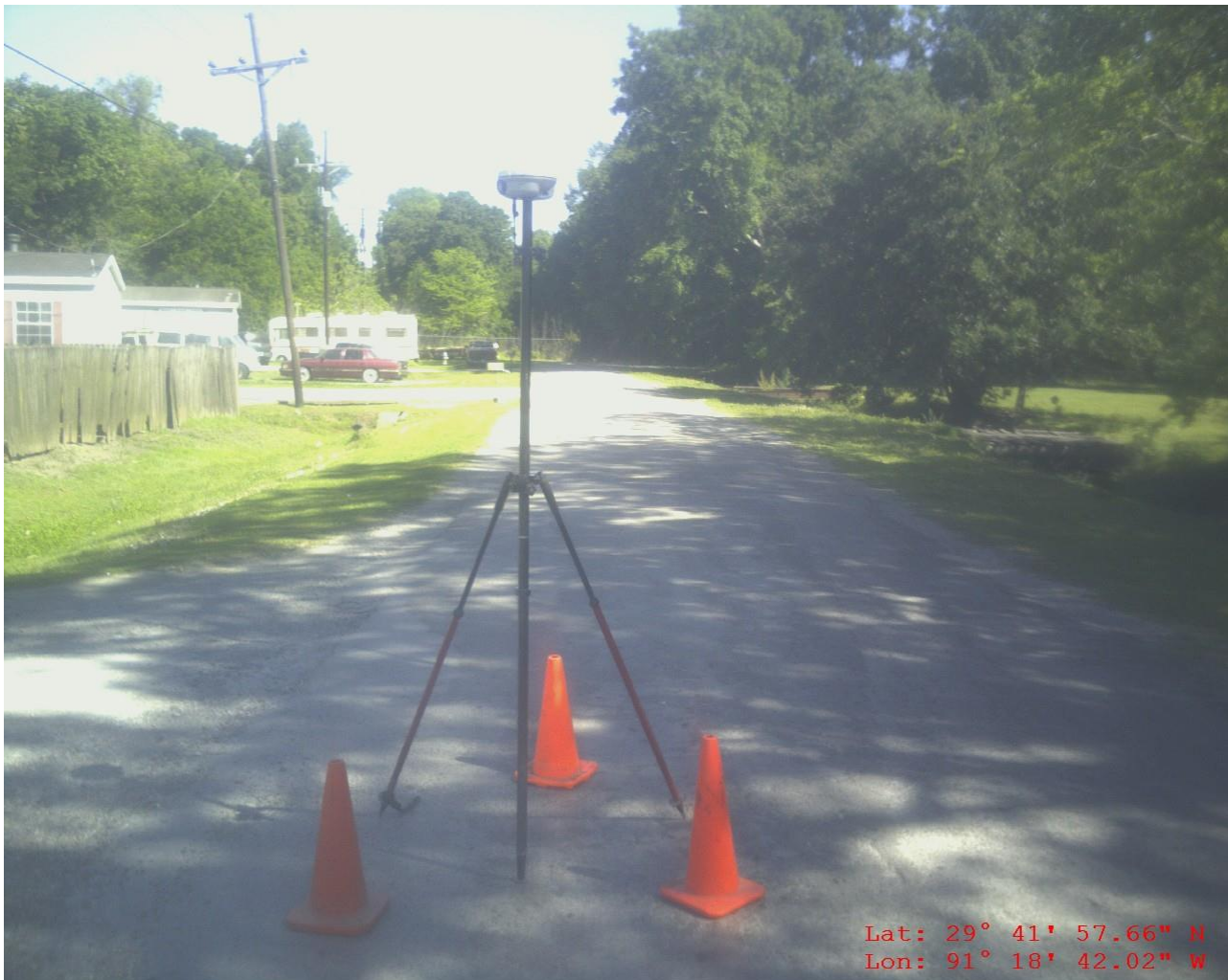
AOI-4 GCP 007 Asphalt road
