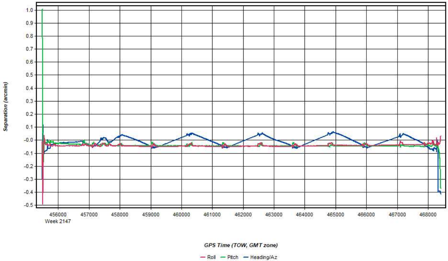
Figure 9: 20210305_062616_3 [Smoothed TC Combined] - Fwd/Rev Attitude Separation Plot
