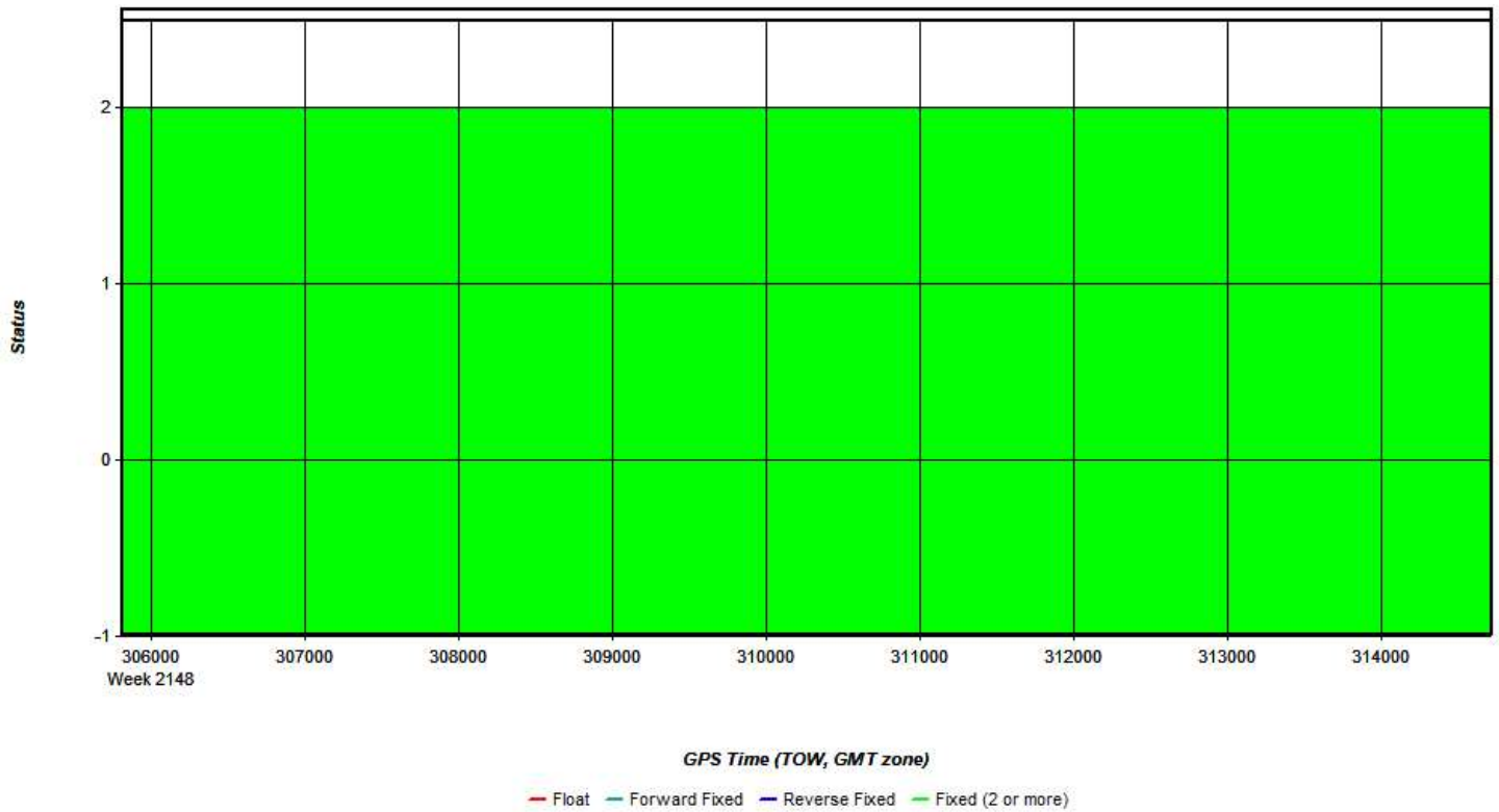
Figure 3: 20210310_125522_6 [Smoothed TC Combined] - Float or Fixed Ambiguity
