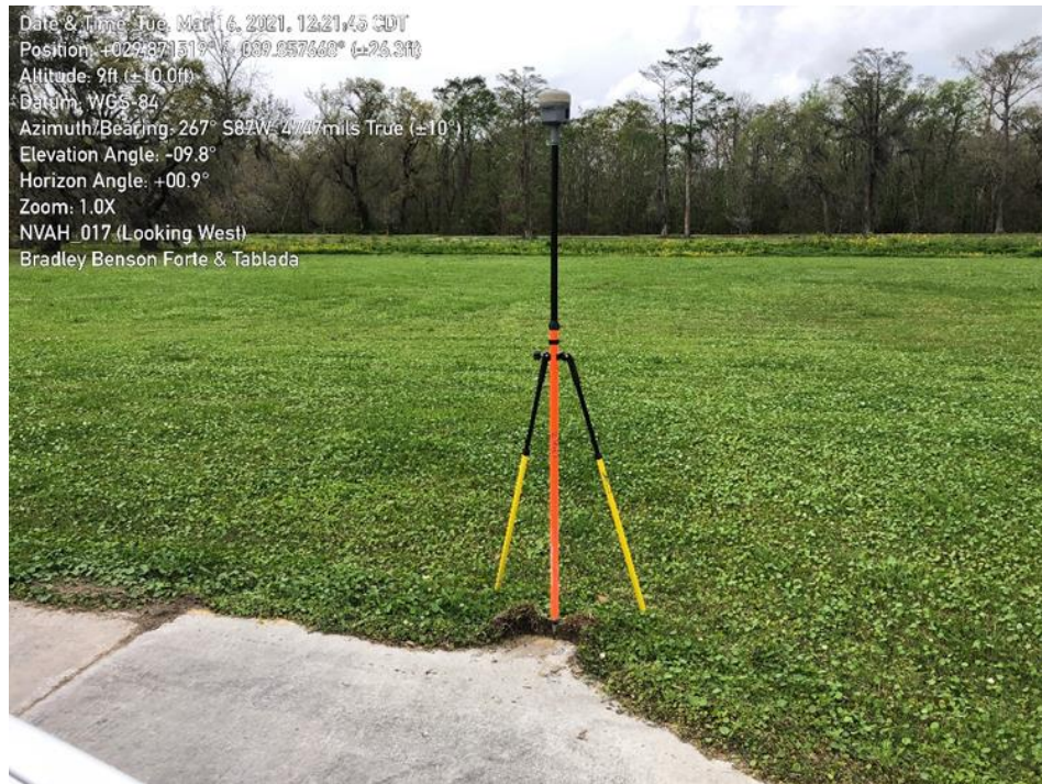
Figure 7. Checkpoint NVA_139. This checkpoint is submerged. Review by Dewberry deemed this survey checkpoint unsuitable to use in the swath vertical accuracy testing.
