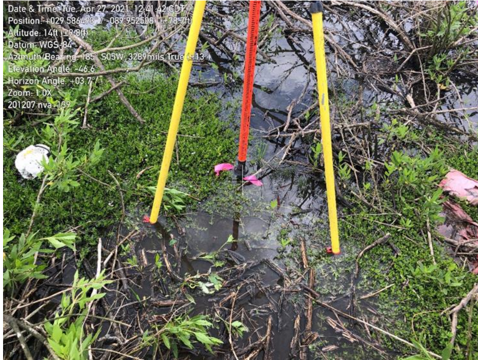
Figure 7. Checkpoint NVA_139. This checkpoint is submerged. Review by Dewberry deemed this survey checkpoint unsuitable to use in the swath vertical accuracy testing.
