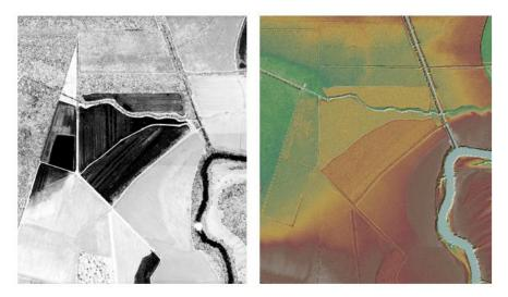
Figure 17 – Tiles15RWQ0994 and 15RWQ0995. All lakes, ponds, irrigated agricultural fields, aquaculture areas and other areas of standing water greater than or equal to 2 acres are included in the delivered breaklines.
