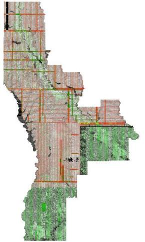
Figure 6– Single return DZ Orthos for the LA Sabine. Inter-swath relative accuracy passes specifications.
