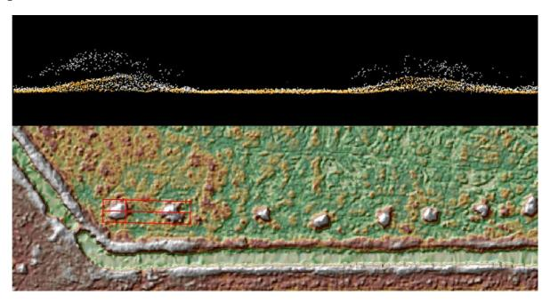
Figure 15 - Tile 15RVP8639. Profile with the points colored by class (class 1=white, class 2=orange) is shown in the top view and a DEM of the surface is shown in the bottom view. These features are correctly included in the ground classification.
