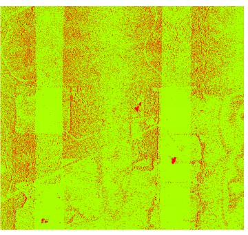
Figure 9– 1-square meter density grid. There are some 1-meter cells that do not contain 2 points per square meter (red areas) due to the irregular spacing of lidar point cloud data. Most 1-square meter cells contain at least 2 points per square meter (green areas) showing there are no systematic density issues. When density is viewed/analyzed by representative 1-square kilometer areas, density passes with no issues.
