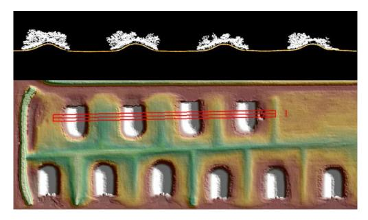
Figure 14 – Tiles 15RVP8539. Profile with the points colored by class (class 1=white, class 2=orange) is shown in the top view and a DEM of the surface is shown in the bottom view. These features are correctly included in the ground classification. LA Sabine River Lidar TO# 140G1018F0025 September 8, 2020 Page 30 of 226
