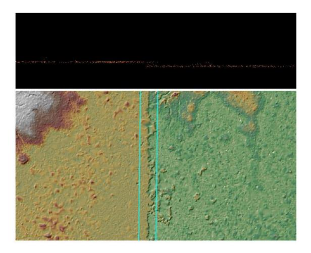
Figure 20– Tile 15RWR0839. An example of a temporal ridge identified by the blue polygon temporal shapefile. Profile with the points colored by class (class 2=orange) is shown in the top view and a DEM is shown in the bottom view.
