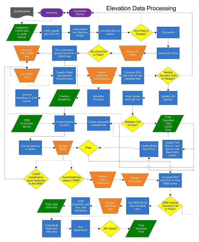
Figure 25-DEM Production Workflow
