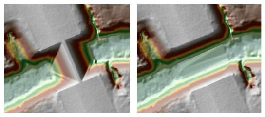
Figure 28-15SVS3602. The DEM on the left shows a bridge saddle artifact while the DEM on the right shows the same location after bridge breaklines have been enforced.
