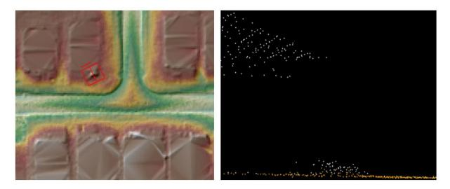
Figure 11 – Tile number 15RVP8438. Profile with points colored by class (class 1=white, class 2=orange) is shown in the right view and a DEM of the surface is shown in the left view. A limited number of these small features are still classified as ground but do not impact the usability of the dataset.
