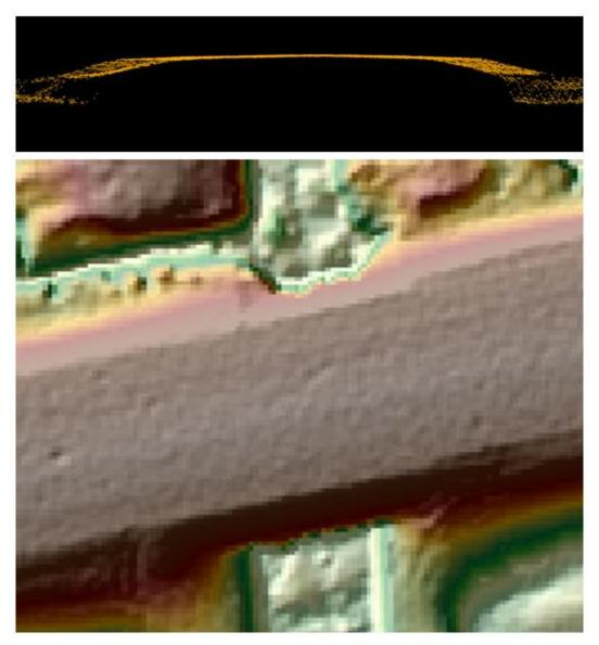
Figure 13– Tile number 15RVP4840. Profile with points colored by class (class 2=orange) is shown in the top view and the DEM is shown in the bottom view. This culvert remains in the bare earth surface. Bridges have been removed from the bare earth surface and classified to class 17.
