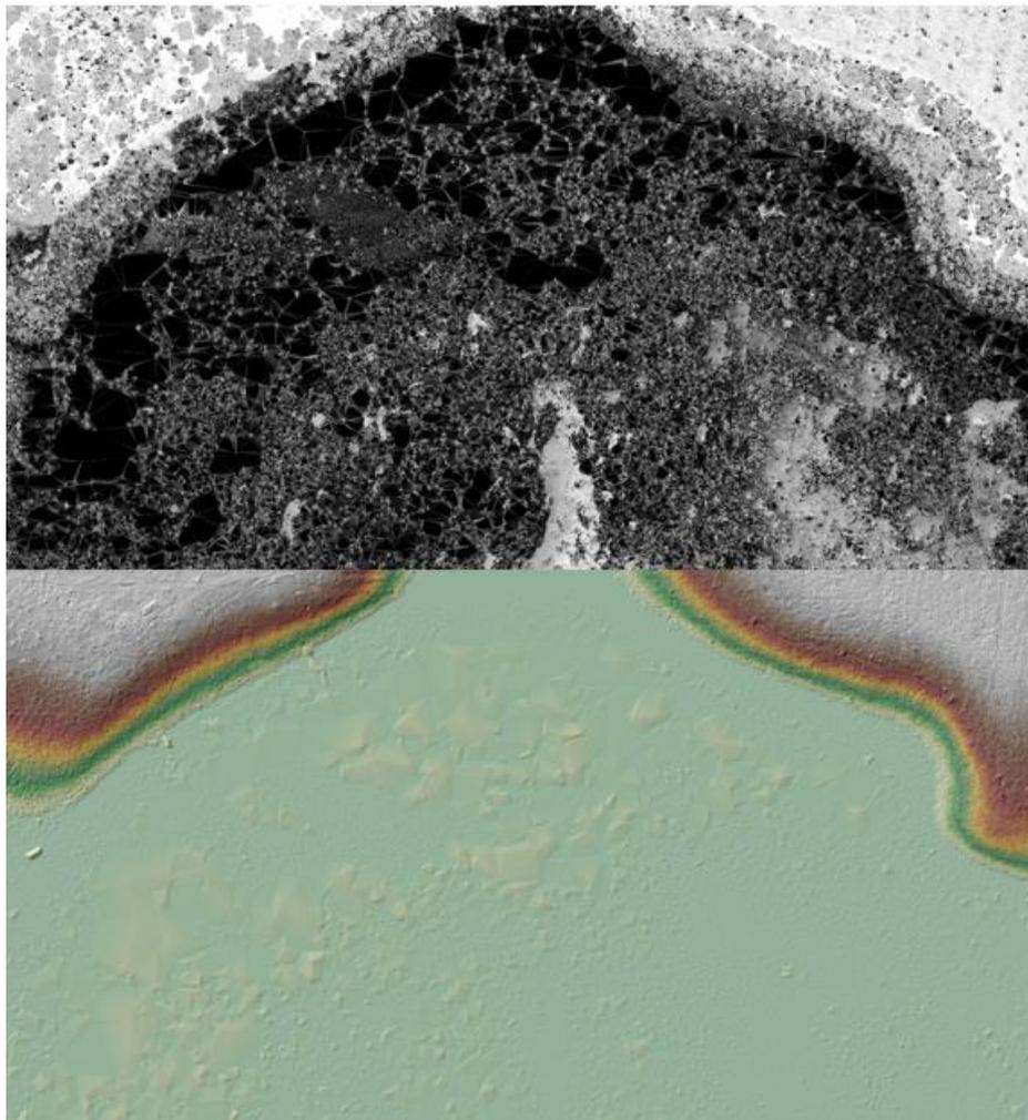
**Figure 19 - Tiles 15RWR0829. The intensity on the top shows a marsh area that was not included in the collected breaklines. The same area is shown in the DEM on the bottom. Due to wet soils and broken terrain, the point density in marsh areas is sparser than surrounding areas and there is more variation in the low points representing ground.**
