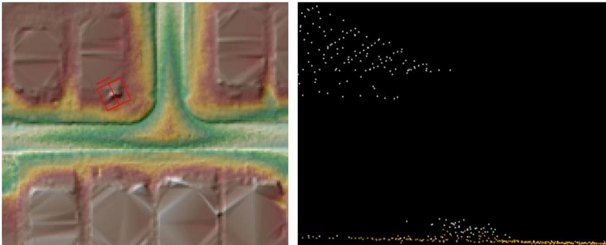
Figure 11 – Tile number 15RVP8438. Profile with points colored by class (class 1=white, class 2=orange) is shown in the right view and a DEM of the surface is shown in the left view. A limited number of these small features are still classified as ground but do not impact the usability of the dataset.
