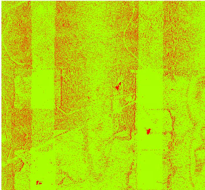
**Figure 9– 1-square meter density grid. There are some 1-meter cells that do not contain 2 points per square meter (red areas) due to the irregular spacing of lidar point cloud data. Most 1-sqaure meter cells contain at least 2 points per square meter (green areas) showing there are no systematic density issues. When density is viewed/analyzed by representative 1-square kilometer areas, density passes with no issues.**
