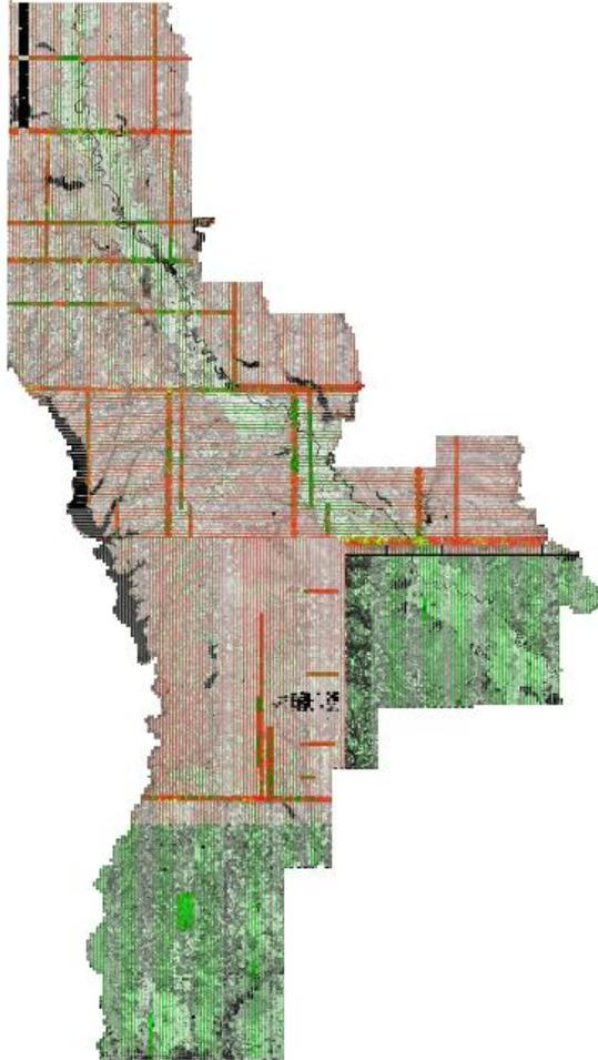
Figure 6– Single return DZ Orthos for the LA Sabine. Inter-swath relative accuracy passes specifications.
