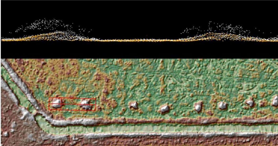
Figure 15 - Tile 15RVP8639. Profile with the points colored by class (class 1=white, class 2=orange) is shown in the top view and a DEM of the surface is shown in the bottom view. These features are correctly included in the ground classification.
