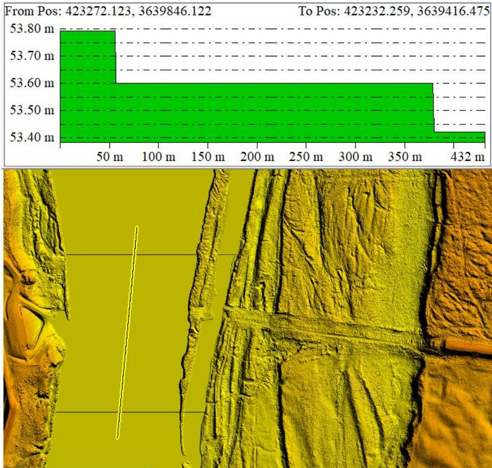
Figure 16 – Tile number 15SVS 2339. Elevation change has been stair stepped. The steps are flat from bank to bank and flow consistently downhill.
