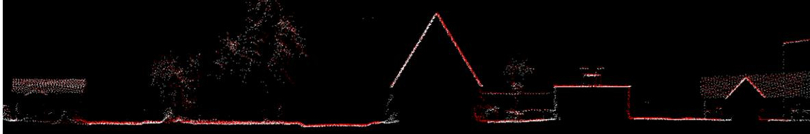
**Figure 8– Horizontal Alignment.** Two separate flight lines differentiated by color (Red/White) are shown in this profile. There is no visible offset between these two flight lines. No horizontal alignment issues were identified.
