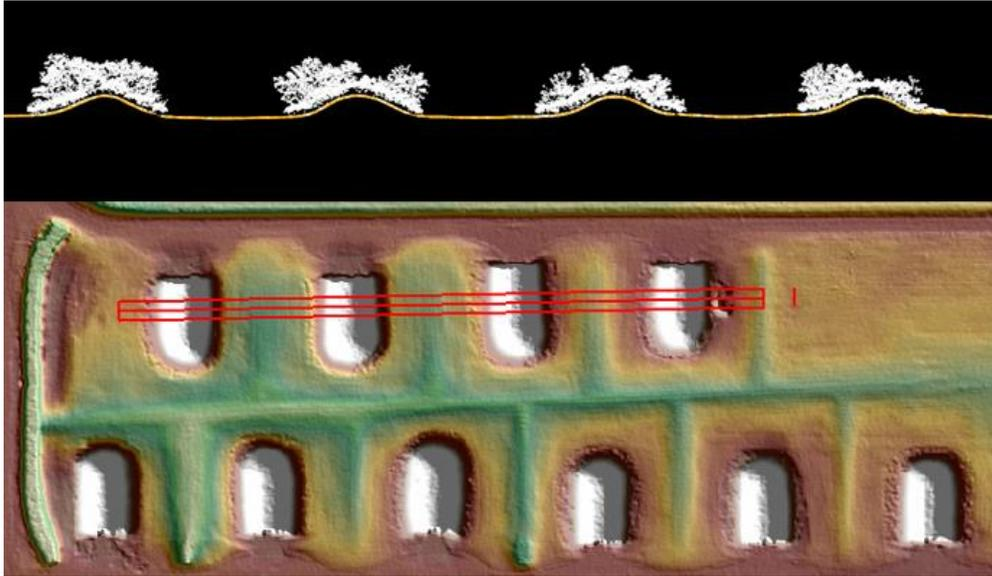
Figure 14 – Tiles 15RVP8539. Profile with the points colored by class (class 1=white, class 2=orange) is shown in the top view and a DEM of the surface is shown in the bottom view. These features are correctly included in the ground classification.
