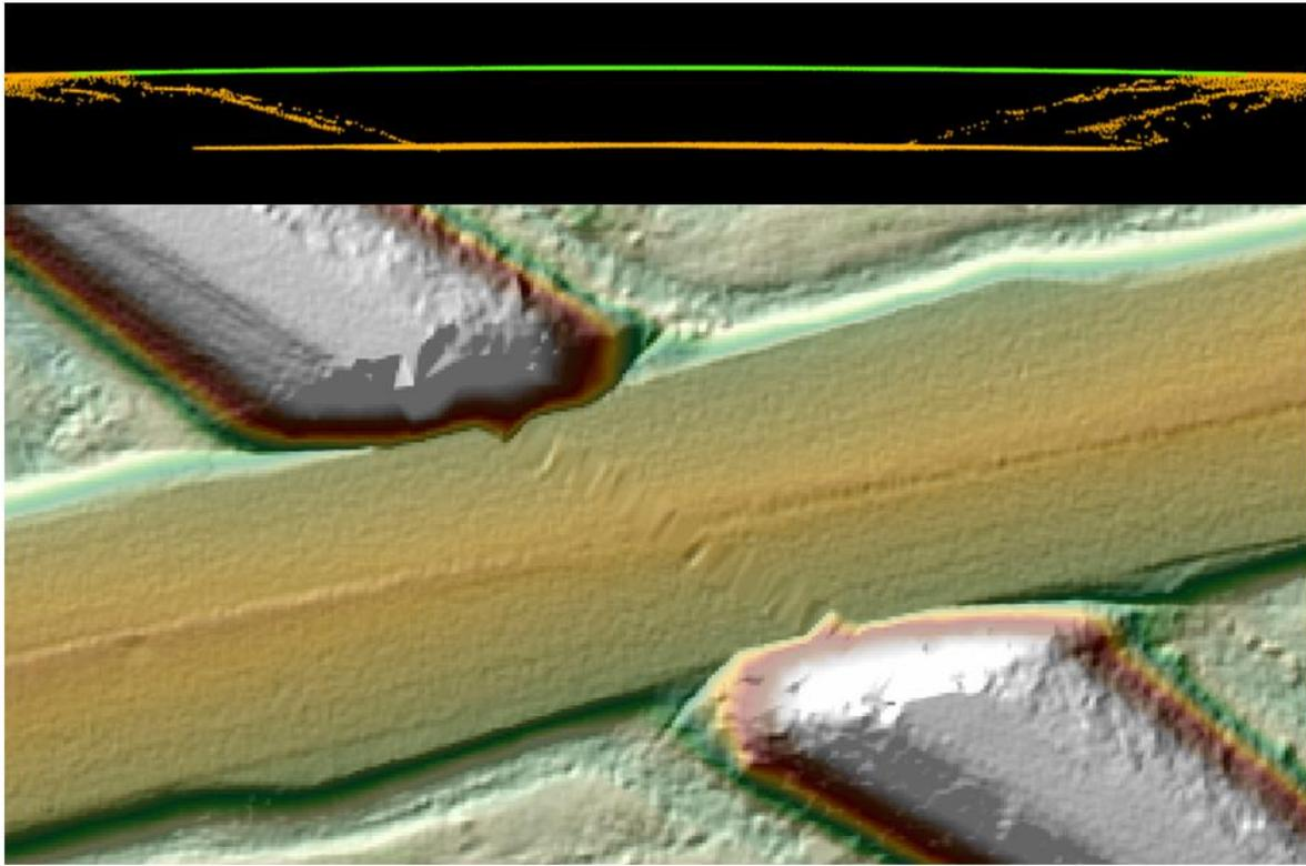
**Figure 12 – Tile number 15RVP5140. The DEM in the bottom view shows an area where a bridge has been removed from ground. The surface model must make a continuous model and in order to do so, points are connected through interpolation. This results in less detail where the surface must be interpolated. The profile in the top view shows the lidar points of this particular feature colored by class. All bridge points (green) have been removed from ground (orange).**
