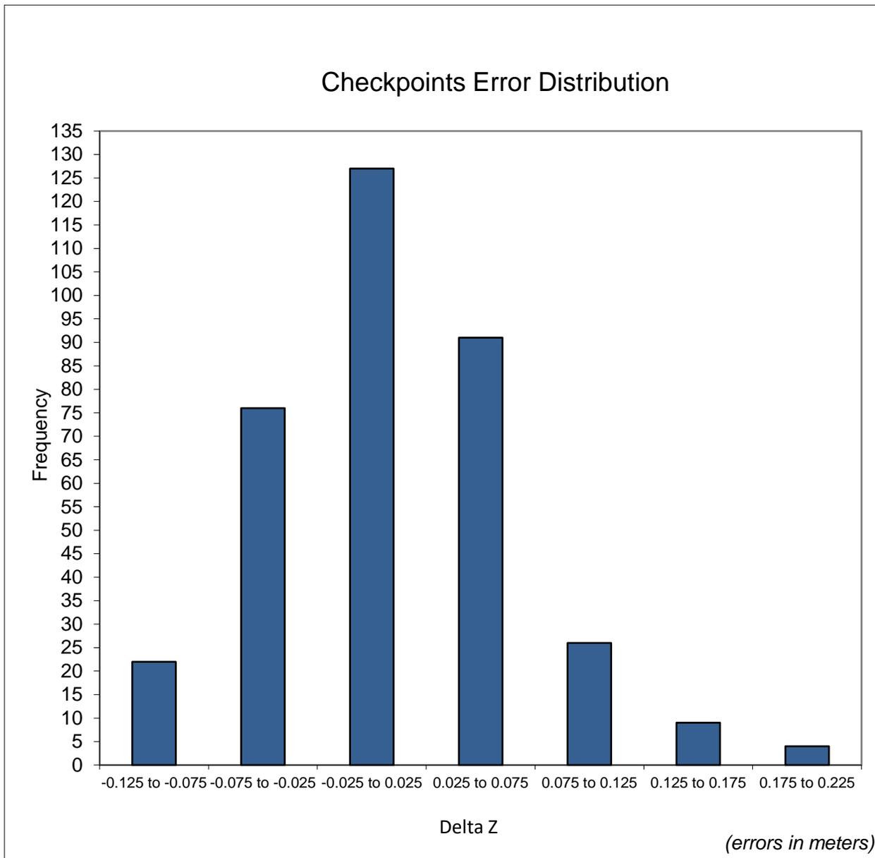
Figure 23 – Histogram of Elevation Discrepancies with errors in meters
