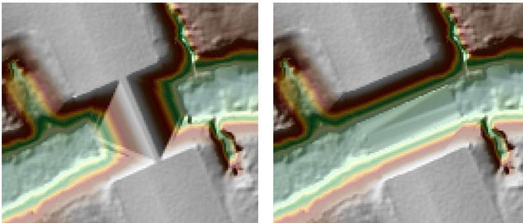
Figure 28-15SVS3602. The DEM on the left shows a bridge saddle artifact while the DEM on the right shows the same location after bridge breaklines have been enforced.
