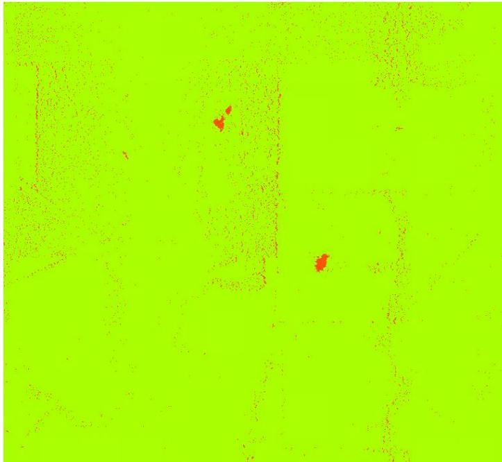
**Figure 10– Spatial Distribution.** All cells (2\*NPS cellsize) containing at least one lidar point are colored green. Cells that do not contain a lidar point, including water bodies which are acceptable NoData area, are colored red. Without removing acceptable NoData areas due to water, 96.3% of cells contain at least one lidar point.
