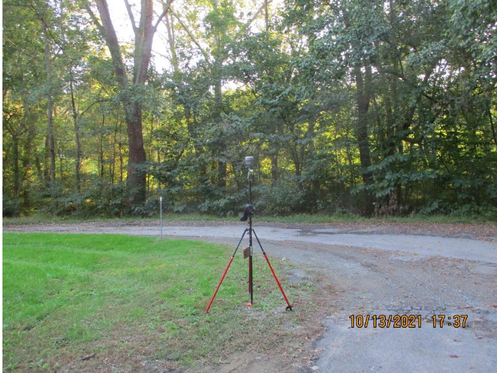
Figure 9. The surveyed elevation of checkpoint VVA_9 is over 4 meters above the ground surface in the lidar data. Review by the surveyor deemed this survey checkpoint erroneous and unsuitable to use in the final vertical accuracy testing.
