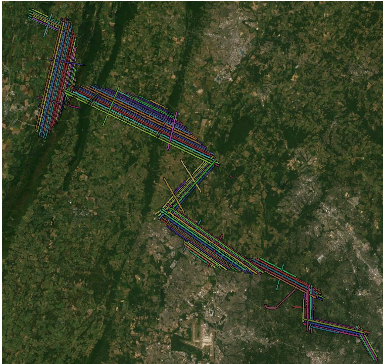
Figure 4 – Lidar swath output showing complete coverage.
