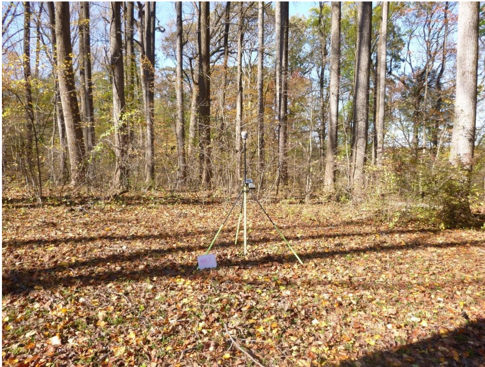
Figure 26 – Checkpoint VVA-7. The surveyed elevation of this forest checkpoint is over 3 meters above the ground surface in the lidar data. Review by the surveyor deemed this survey checkpoint erroneous and unsuitable to use in the final vertical accuracy testing.
