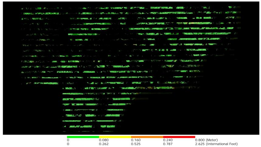
A maximum vertical separation cutoff has been applied to this graphic for the purpose of masking out disruptive features that do not show calibration issues between flight lines (e.g., trees, moving cars, etc.).
