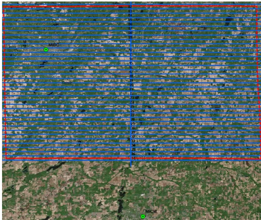
Figure 2.5: Acquired LiDAR Flight Lines/Base Station Locations
