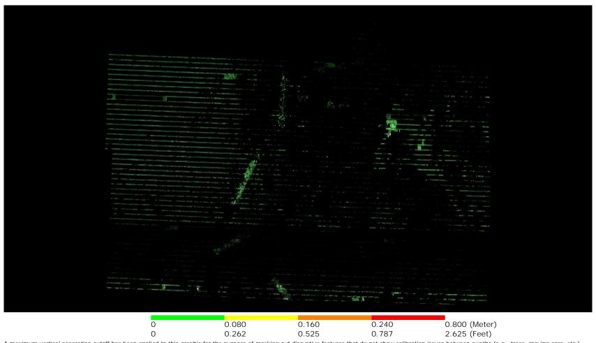
A maximum vertical separation cutoff has been applied to this graphic for the purpose of masking out disruptive features that do not show calibration issues between swaths (e.g., trees, moving cars, etc.).
