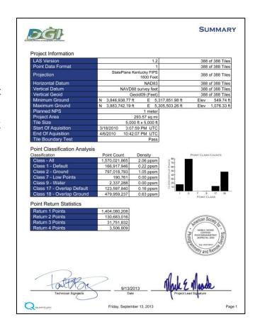
all tiles in the delivery. A quick test is also performed to verify that all points within a tile fit within the exact boundary of the tile. This is shown as the tile boundary test and is presented in terms of a pass/fail. If any points for an individual tile are found outside of the logical tile boundary, an exception log is created that includes the tile name and the horizontal location and vertical position of all exceptions within that tile.
