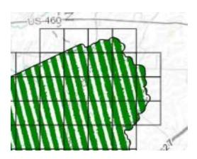
throughout parallel flight lines. Significant changes in terrain elevations, turbulence that can affect the roll of the aircraft during acquisition, the pilot's ability to follow preplanned flight paths at consistent altitudes, and sensor performance will all result in variation within this overlap.
