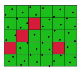
within that grid cell as indicated in the graphic at right. If at least one return falls within a cell then that cell is counted as a populated cell. If not, that cell is counted as one void of returns. If hydro breaklines were collected for the project then any cell that either
