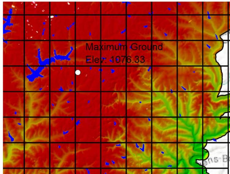
shaded and therefore appear as a void area within the graphic), and can also illustrate large data gaps within individual tiles. The location of the minimum and maximum points within the ground class are also located on this graphic.
