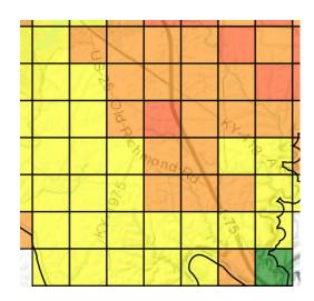
surfaces (e.g., fresh asphalt). If the project boundary splits any tile, the calculation takes place only within the project boundary. Translucent colors are used in this graphic so that you can see the project map behind the rendering. This can be useful in evaluating tiles with lower first return point densities that might be affected by water bodies that are often visible in the background project map.
