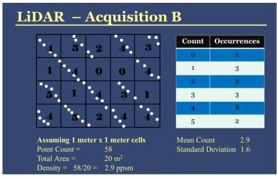
along- and cross-track point spacing is fairly consistent, indicating an effective flight plan. In Acquistion B, the cross track point spacing is much tighter (nominally about a 4 to 1 ratio) than the along track spacing, which would be undersirable for most LiDAR projects. Note that the nominal point density is exactly the same for both at 2.9 ppsm. The standard deviation, however, is considerably higher for Acquisition B.
