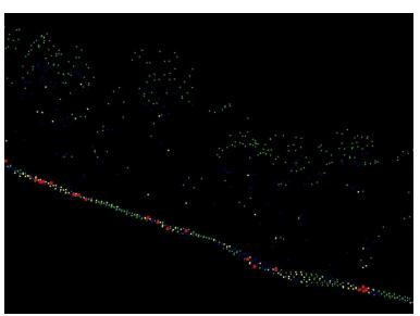
fourth returns within each of these cells and then render the project area based on these densities. Cells with a very low density of these multiple returns will appear transparent. Cells with high densities will be rendered as darker colors.
