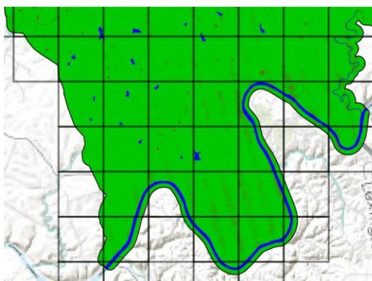
The USGS specification defines data voids within a single swath as unacceptable, except when caused by water bodies, areas of low near infra-red reflectivity such as asphalt or composition roofing, or where filled in by another swath. It is extremely rare for this void test to result in no voids within a dataset, but the location of the voids are almost always found in small streams or ponds that are less than the collection requirements for hydro bodies, or in fresh asphalt surfaces.
