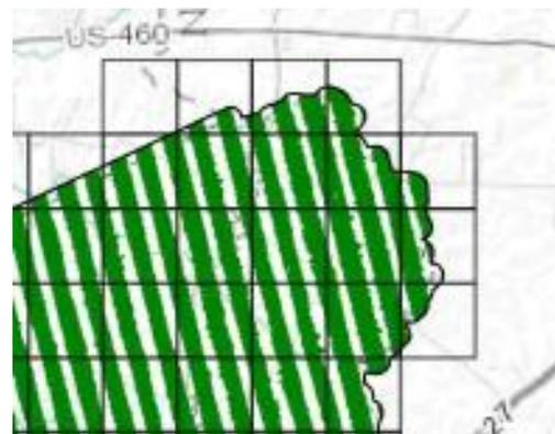
throughout parallel flight lines. Significant changes in terrain elevations, turbulence that can affect the roll of the aircraft during acquisition, the pilot's ability to follow pre-planned flight paths at consistent altitudes, and sensor performance will all result in variation within this overlap.
