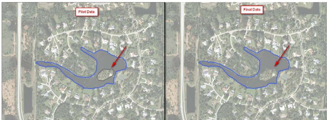
Figure 7 Missing Island from Lake
