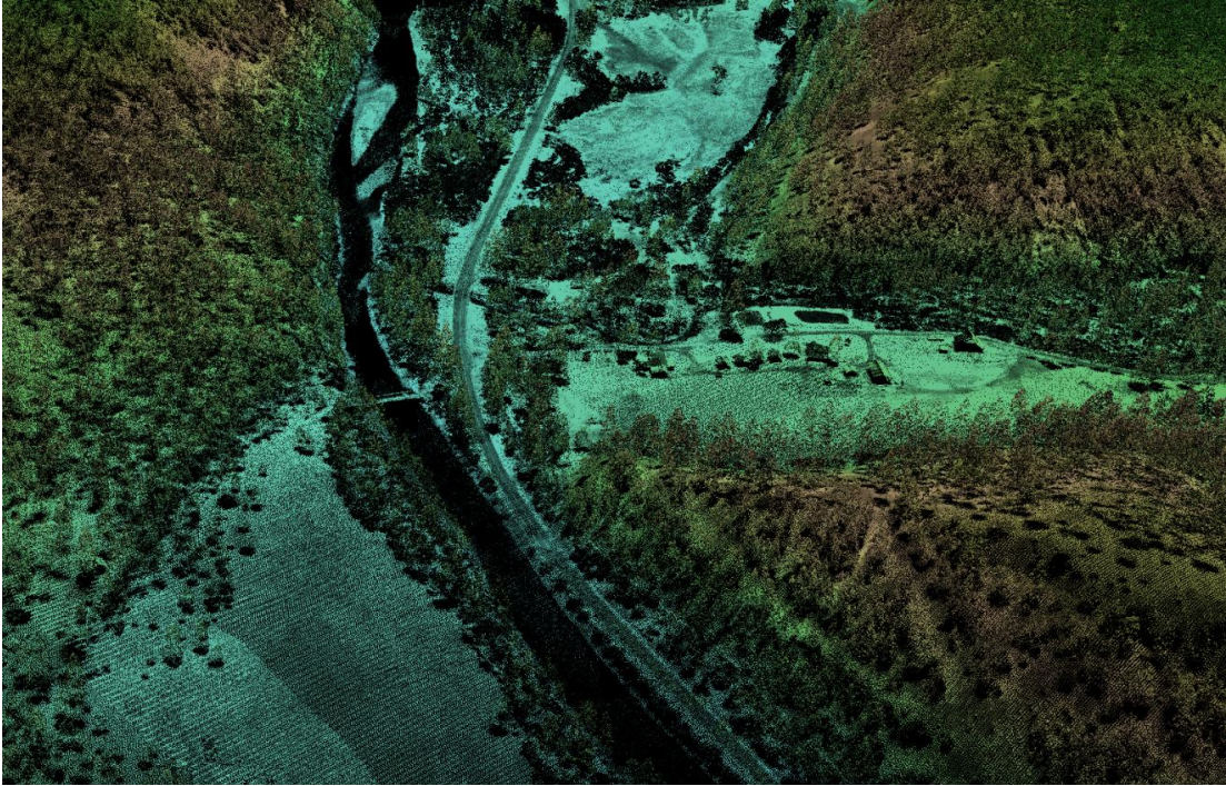
Figure 10. 3D views of LiDAR point clouds colored by elevation and shaded by intensity. Top image looking Northwest at the confluence between Trapper creek and West Fork Bitterroot River along Fork Road. Bottom image looking east at the confluence of Saint Clair Creek (left hand side) and Gird Creek (right hand side).
