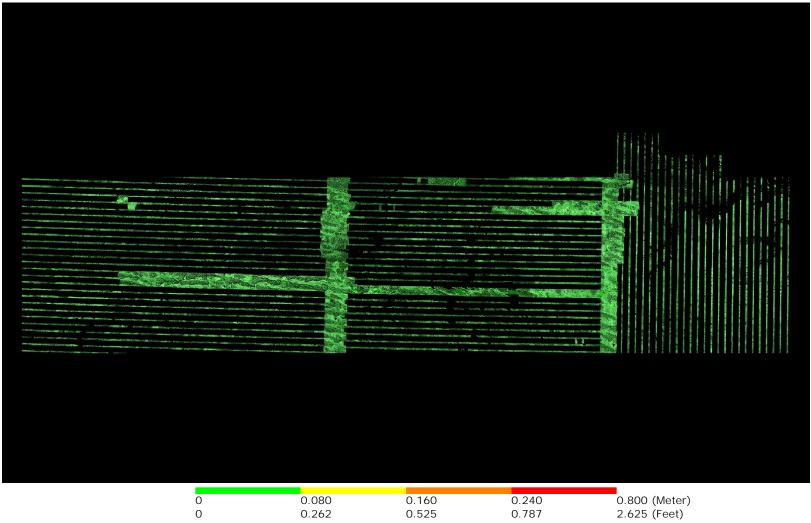
A maximum vertical separation cutoff has been applied to this graphic for the purpose of masking out disruptive features that do not show calibration issues between swaths (e.g., trees, moving cars, etc.).
