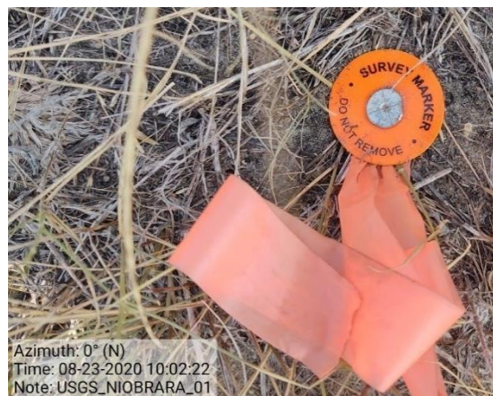
Figure 4: NV5-established monument USGS_NIOBRARA_01
