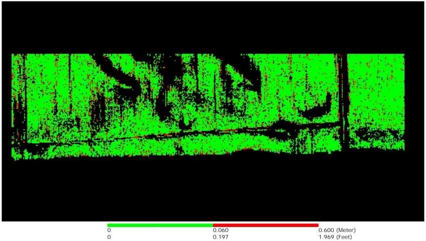
A maximum vertical separation cutoff has been applied to this graphic for the purpose of masking out disruptive features that are not applicable for depicting sensor noise within individual swaths (e.g., trees, moving cars, etc.).
