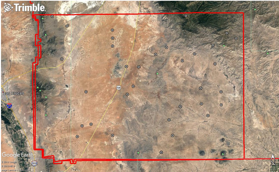
Figure 4: Vegetated Vertical Accuracy (VVA) Point Distribution
