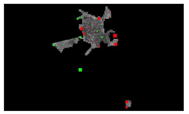
Green represents where the lidar surface is above the check point (positive elevation error).
