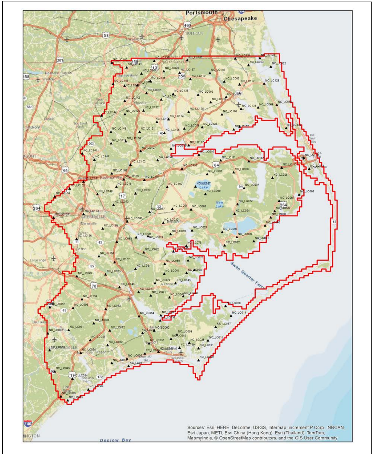
Figure 5 LiDAR Ground Control Points Used in Calibration
