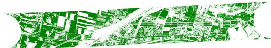
Figure 2 Vertical difference between forward and backward scan at 1000 m AGL.
