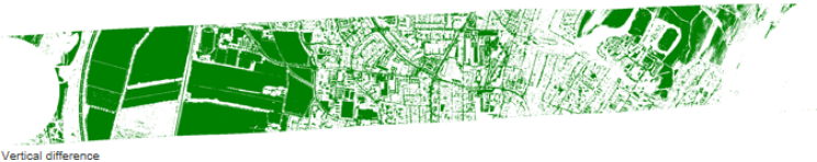
Figure 2 Vertical difference between forward and backward scan at 1000 m AGL.
