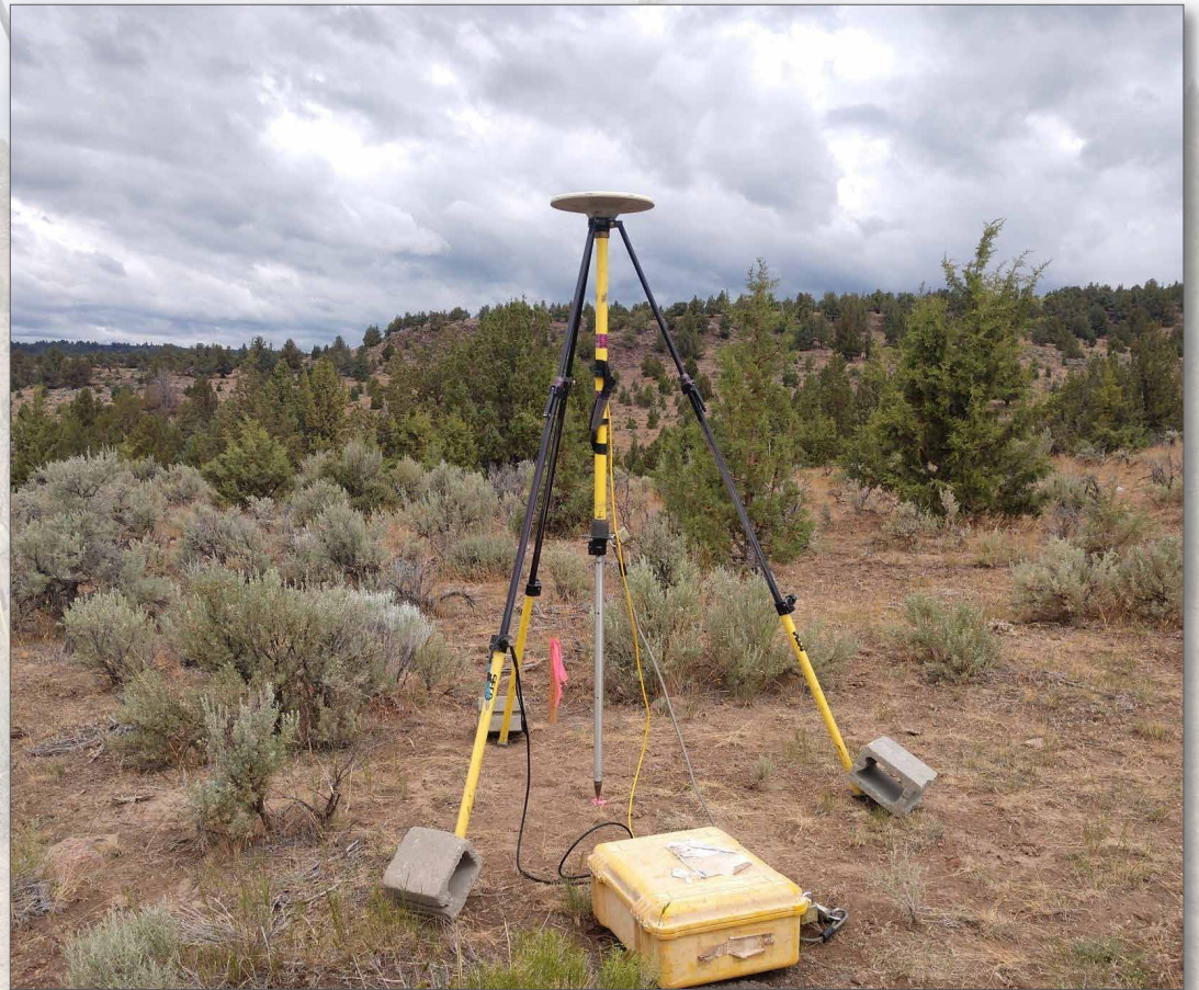
Figure 2: Zephyr GNSS Geodetic Model 2 antenna set up over Silver_Creek_04 monument
