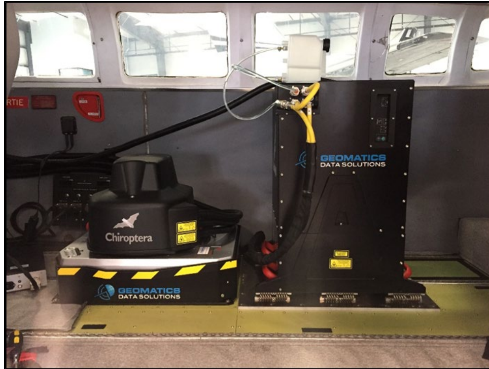
Figure 4: Hawkeye 4X Bathymetric Lidar Sensor Installation
