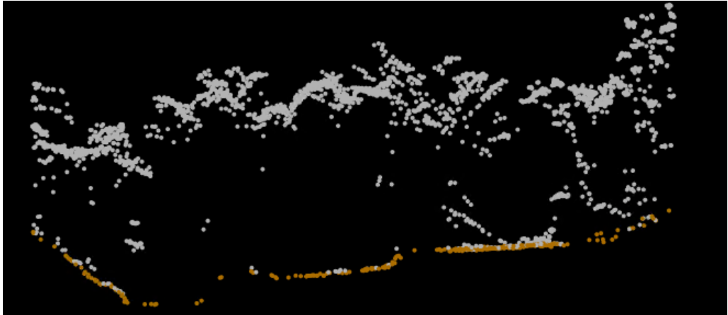
Figure 15: Cross Section from the 2016 LiDAR collection showing vegetative structures and respective heights. The profile width is 3 meters.
