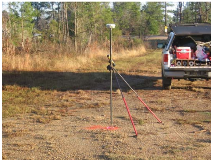
80D MAG NAIL SET IN GRAVEL AREA, 27' NORTH OF HARPER STREET AND 50' WEST OF S. PEARSON ROAD
