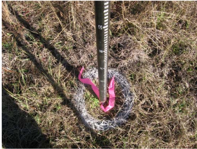
80D NAIL SET ON NORTH SIDE OF COUNTY LINE ROAD (12' N. OF EDGE OF PAVEMENT)
