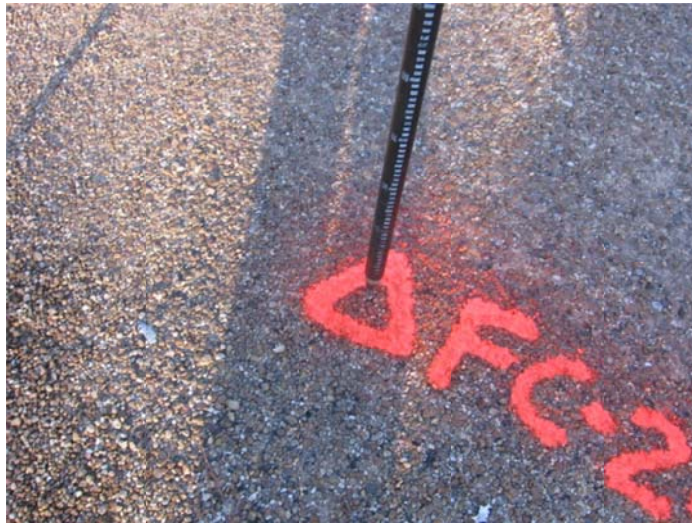
PK NAIL @ CL INTERSECTION OF PEACOCK ROAD AND MAIN STREET
