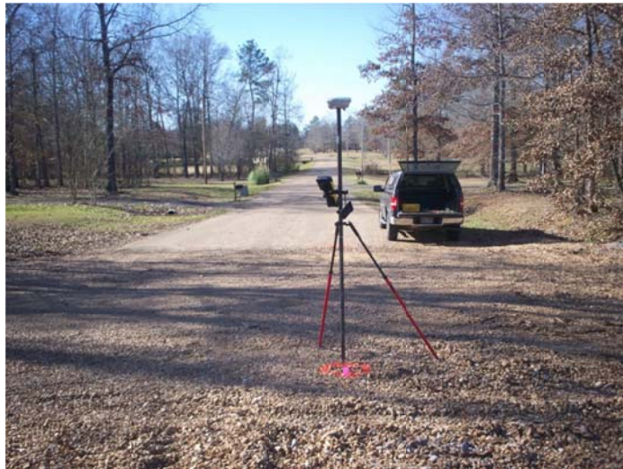
80D MAG NAIL SET 33' FROM EDGE OF GRAVEL IN THE CENTER OF THE GRAVEL AREA
