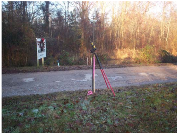
80D NAIL SET 2' EAST OF EDGE OF ROCK ROAD AND 50' SOUTH OF POWER POLE
