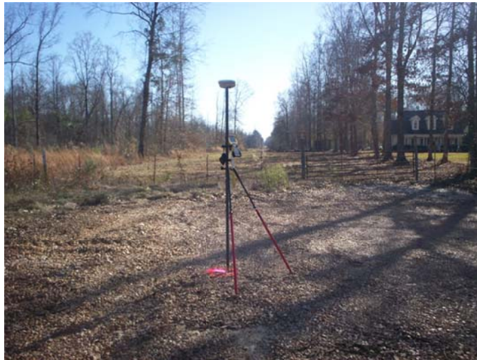
80D MAG NAIL SET 33' FROM EDGE OF GRAVEL IN THE CENTER OF THE GRAVEL AREA
