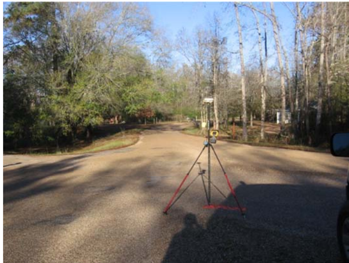
PK NAIL @ CL INTERSECTION OF PEACOCK ROAD AND MAIN STREET
