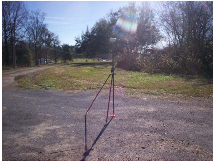
80D NAIL SET IN CENTER OF ASPHALT CUL-DE-SAC – 68' FROM EDGE OF GRAVEL DRIVE
