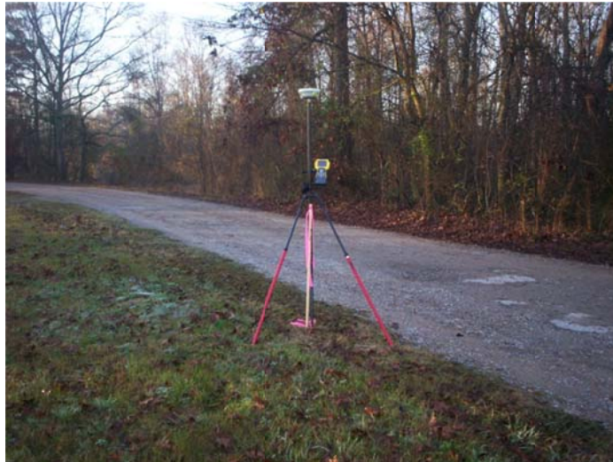
80D NAIL SET 2' EAST OF EDGE OF ROCK ROAD AND 50' SOUTH OF POWER POLE
