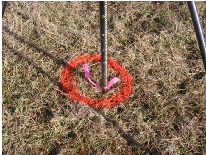
80D NAIL SET ON THE SOUTH SIDE OF FLORENCE TO BYRAM ROAD IN OPEN AREA
