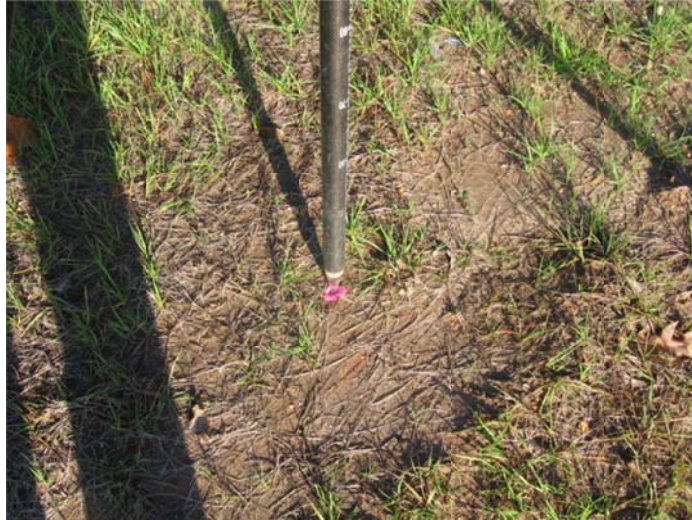
80D MAG NAIL IN MOWED LAWN ON WHITE ROAD (HOUSE # 712), 27' WEST OF ROAD
