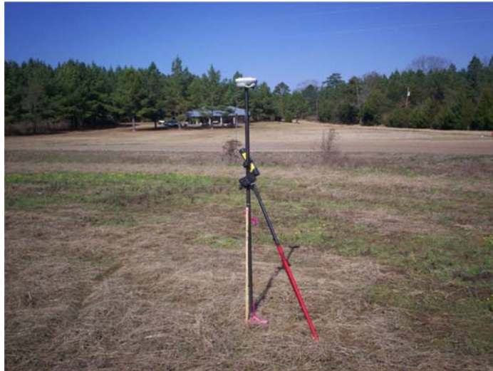
80D NAIL SET IN FIELD 139' SOUTH OF CL OF OLD HWY43 – 88' WEST OF CL OF WILSON-BATES ROAD
