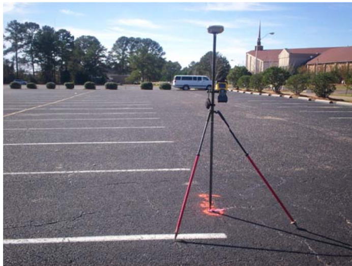
80D MAG NAIL SET 39' SOUTH EDGE OF ASPHALT PARKING LOT AND 44' WEST OF PARKING LOT EDGE
