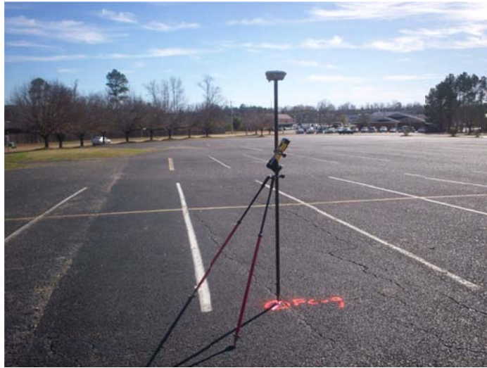
80D MAG NAIL SET 39' SOUTH EDGE OF ASPHALT PARKING LOT AND 44' WEST OF PARKING LOT EDGE
