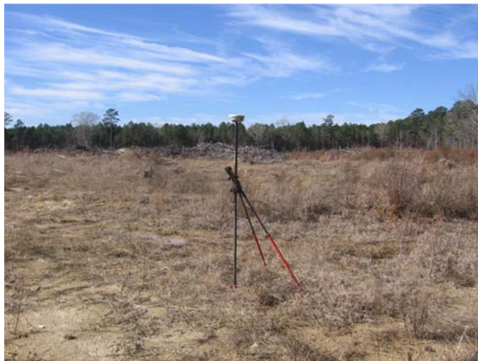
80D NAIL SET IN CUTOVER - 64' WEST OF SHELL OIL ROAD – 20' EAST OF DISTRIBUTION LINE
