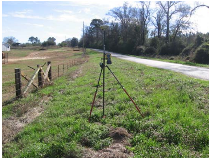
80D NAIL SET IN OPEN AREA – 10' FROM EDGE OF PAVEMENT OF WOODS ROAD
