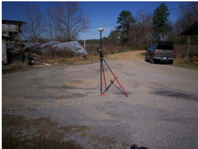
80D NAIL SET IN CENTER OF ASPHALT CUL-DE-SAC – 68' FROM EDGE OF GRAVEL DRIVE
