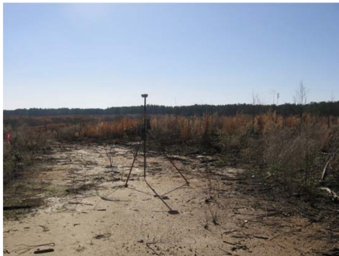
80D NAIL SET IN CL OF DIRT WOODS ROAD IN AREA OF CUTOVER TIMBER – 60' SOUTH OF HEAD-NEELEY ROAD
