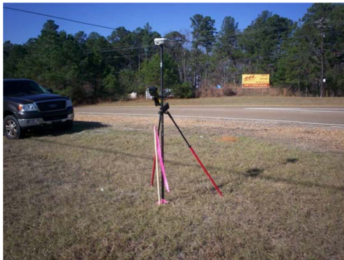
80D MAG NAIL SET 77' SOUTH OF CL OF OLD HWY 71 AND 136' WEST OF SOUTH BOUND LANE OF HWY 71
