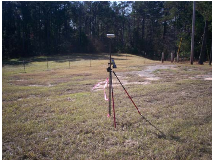
80D MAG NAIL SET 77' SOUTH OF CL OF OLD HWY 71 AND 136' WEST OF SOUTH BOUND LANE OF HWY 71
