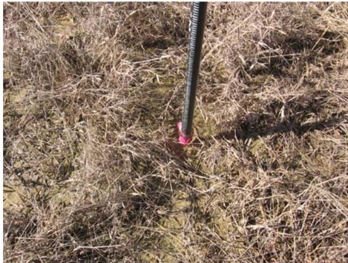
80D NAIL SET IN CUTOVER - 64' WEST OF SHELL OIL ROAD – 20' EAST OF DISTRIBUTION LINE
