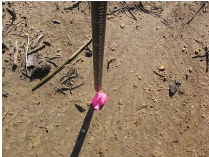
80D NAIL SET IN CL OF DIRT WOODS ROAD IN AREA OF CUTOVER TIMBER – 60' SOUTH OF HEAD-NEELEY ROAD
