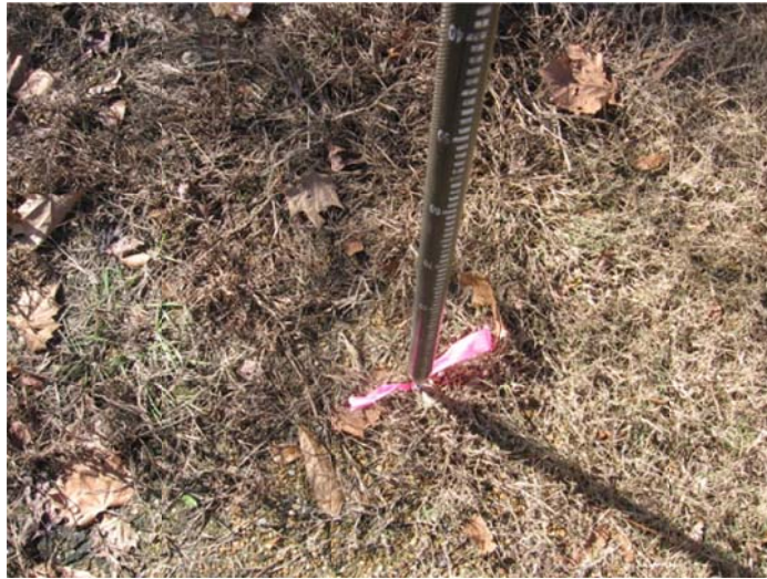
80D NAIL SET 10' WEST OF JOHNS SHILOH ROAD @ PULLOFF AND GROWN OVER FIELD
