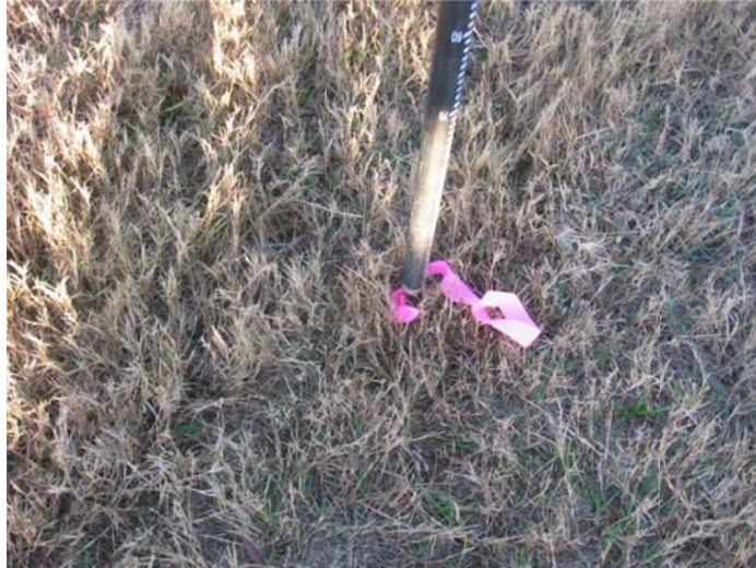
80D NAIL SET 7' EAST OF EAST EDGE OF ASPHALT HWY 541 - 30' SOUTH OF CL OF PAUL CRAFT DRIVE
