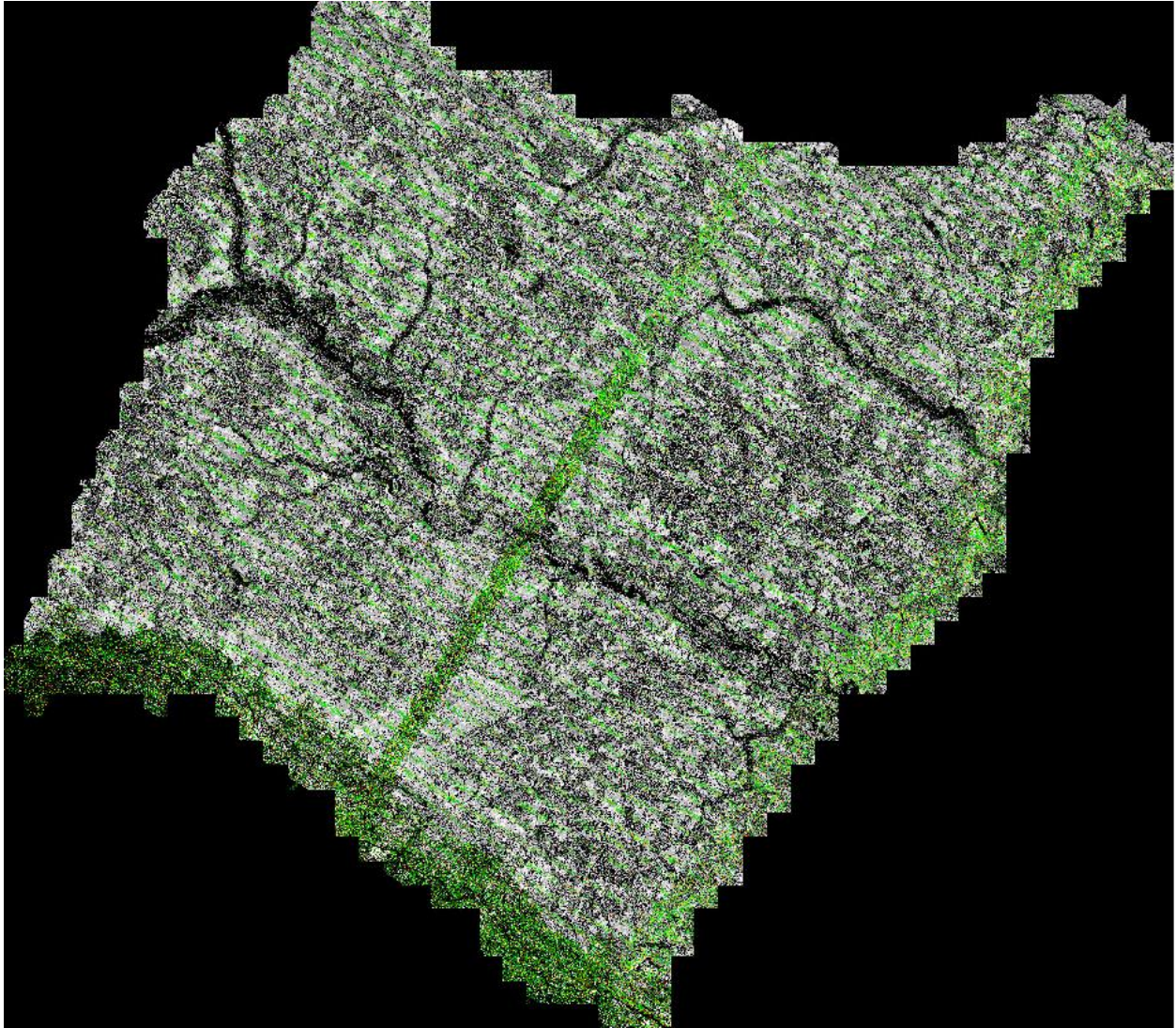
Figure 5 - Single return DZ Orthos for the South Carolina Williamsburg County. Inter-swath relative accuracy passes specifications.
