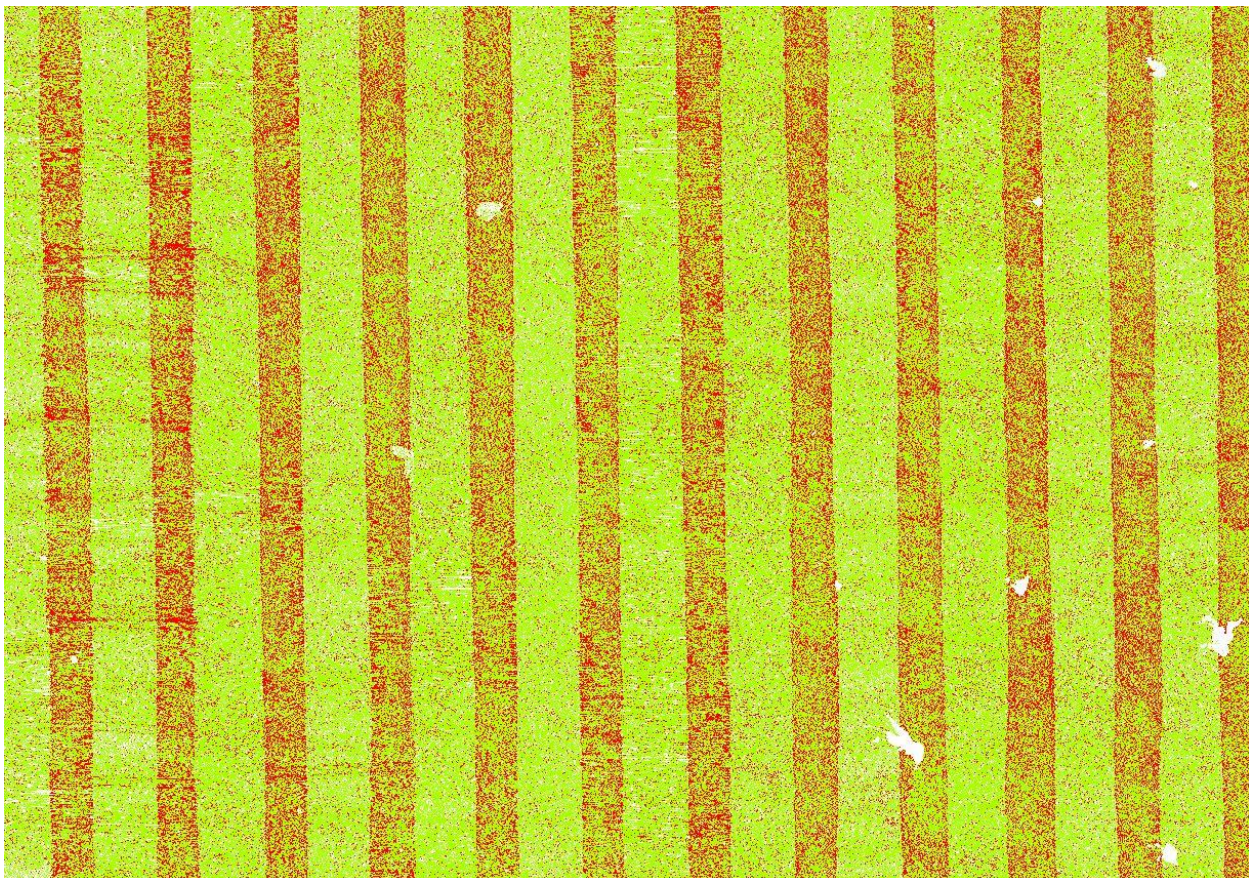
Figure 5. Intra-swath relative accuracy. The top image shows the entire project area; flat, open areas are colored green as they are within 6 cm whereas sloped terrain is colored red because it exceeds 6 cm maximum difference, as expected, due to actual slope/terrain change. The bottom image is a close-up of a flat area. With the exception of vegetated areas (shown as red speckling/mottling as the elevation/height difference in vegetated areas will exceed 6 cm) and swath sidelap/overlap (red striping), this open flat area is acceptable for repeatability testing. Intra-swath relative accuracy passes specifications.
