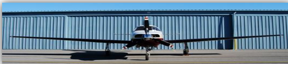
Exhibit 9: The imagery acquisition platform for the Santa Fe County project was a Piper PA-46 Malibu. With a maximum cruise speed of 213 knots, our Malibu provided quick mobilization to and acquisition of the areas of interest.
