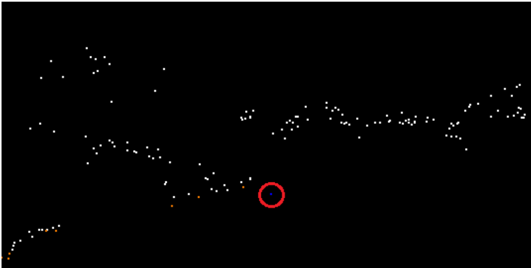
Figure 14- The above image shows the LiDAR cross section of FO-05. FO-05 was located on a hill under tree cover where LiDAR could not penetrate to the bare earth surface.
