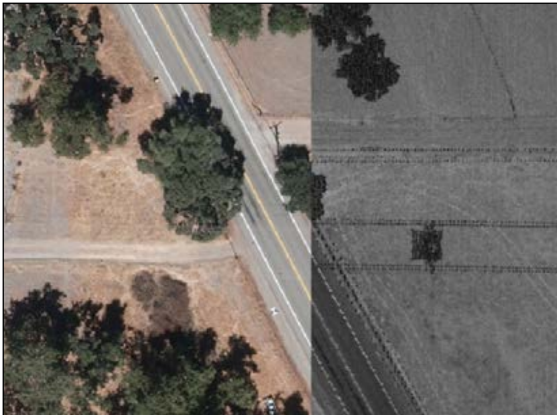
Example of co-registration of color images with LiDAR intensity images.
