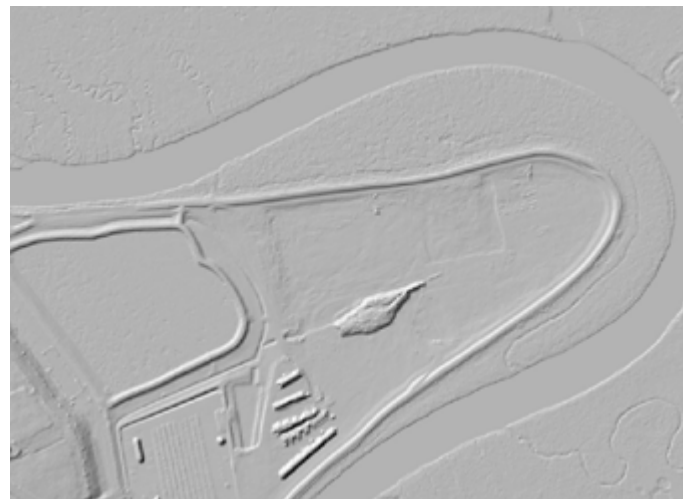
Examples of bare-earth hydroflattened DEMs along the Petaluma River in Delivery Area One of the Sonoma County Project Area
