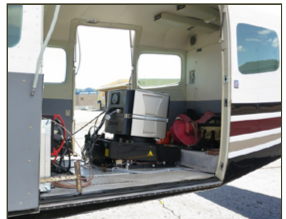
Below: UltraCam Eagle installed in the aircraft.
