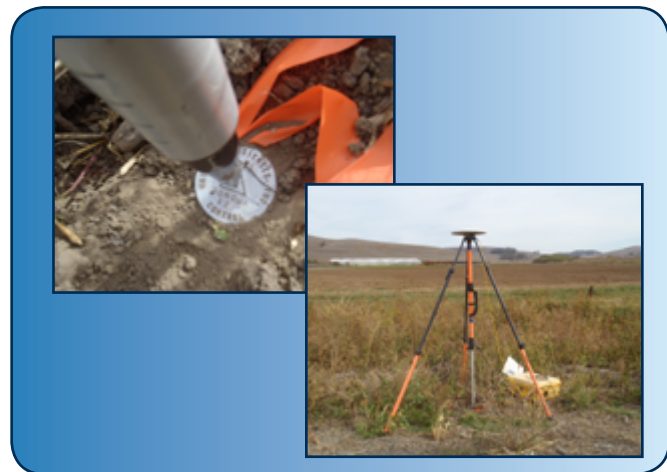
Above: Sonoma_12 survey cap and accompanying R7 Base Station.
