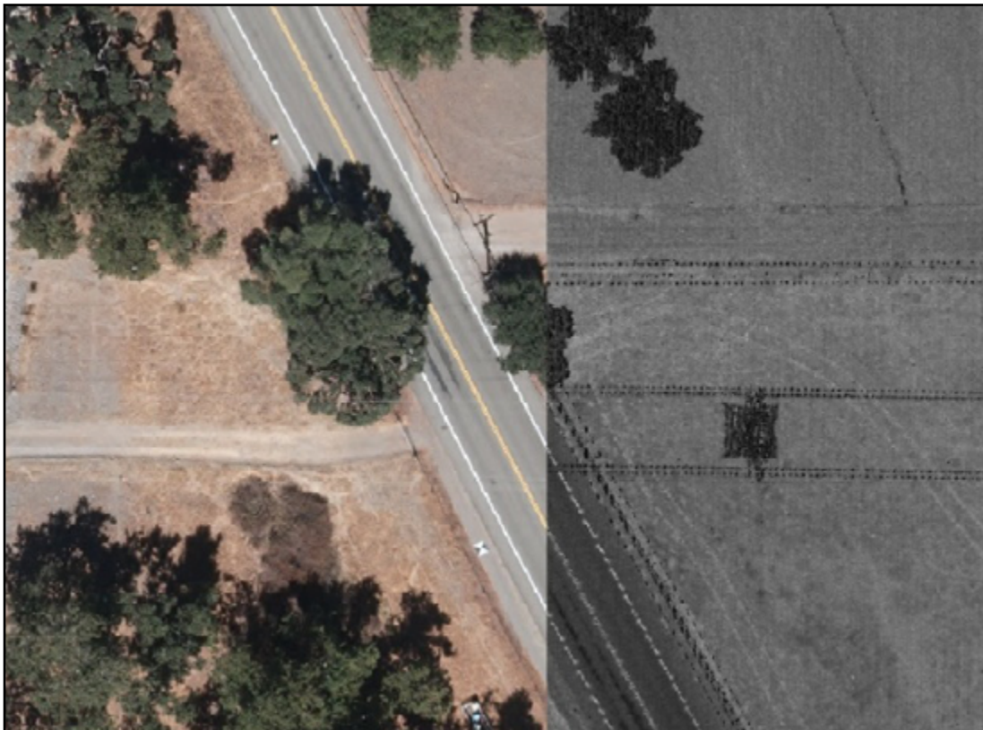
Above: Example of co-registration of color images with LiDAR intensity images.
