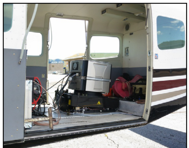
Below: UltraCam Eagle installed in the aircraft.
