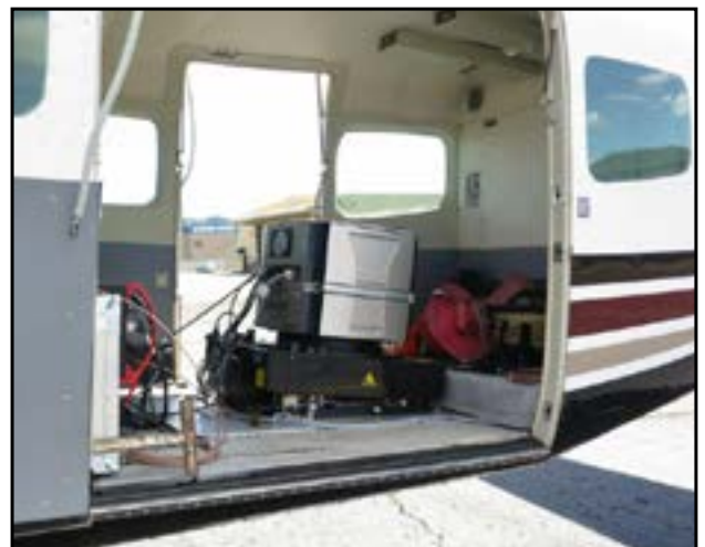
Below: UltraCam Eagle installed in the aircraft.
