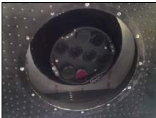
UltraCam Eagle lens configuration as viewed from the Cessna Caravan.
