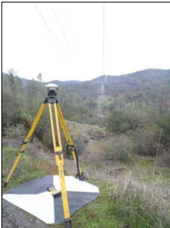
Above: WSI painted permanent air target. Below: WSI temporary air target.
