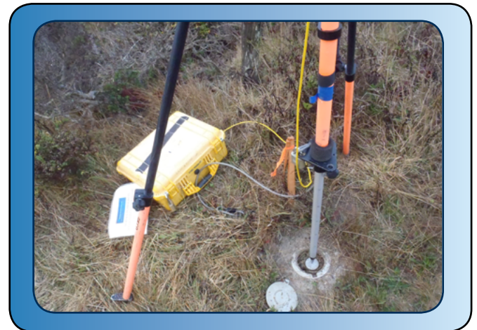
JT9623 survey cap and accompanying R7 Base Station.
