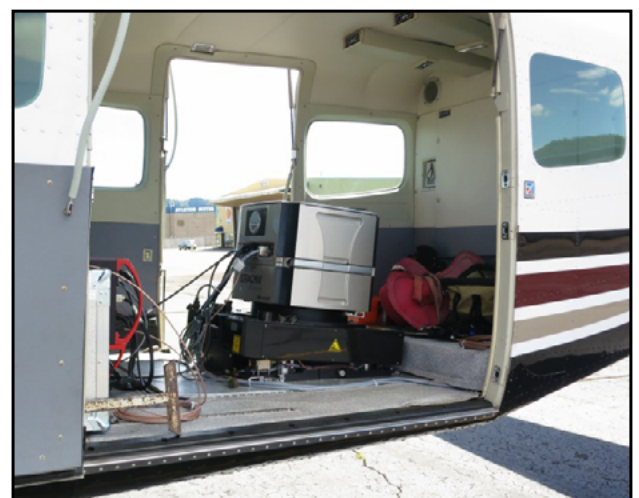
Below: UltraCam Eagle installed in the aircraft.
