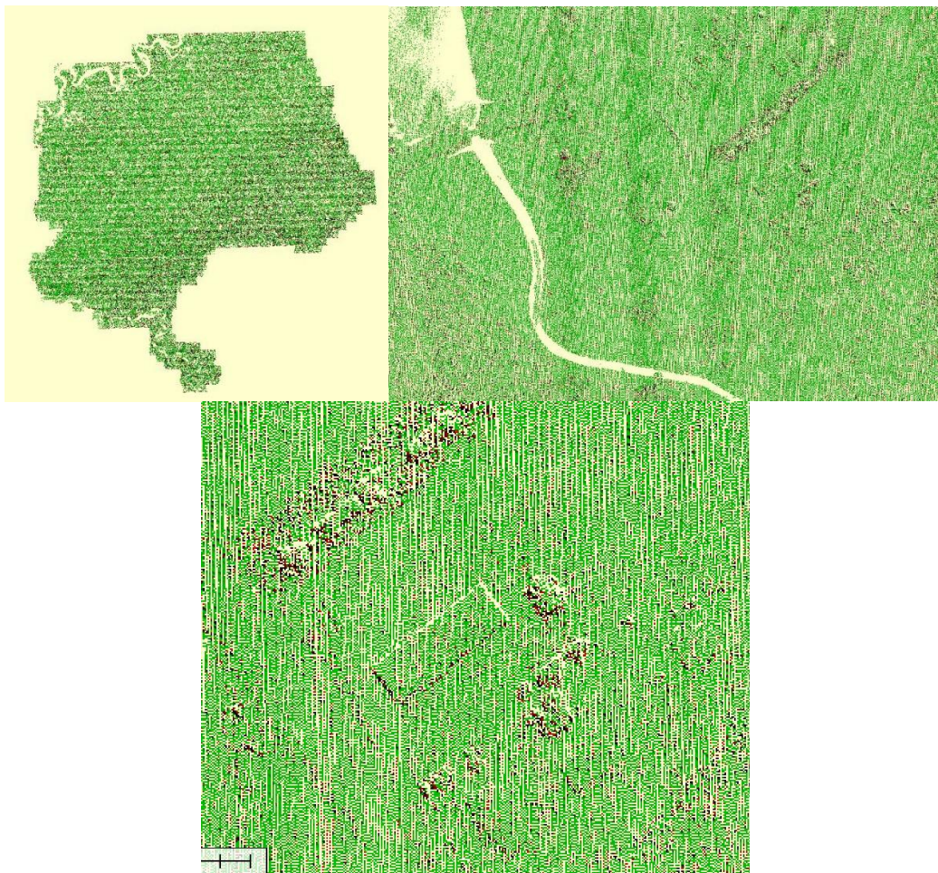
Figure 6–Intra-swath relative accuracy. The top left image shows the full project area; areas where the RMSD_z is \leq 6 cm per pixel within each swath are colored green and areas exceeding 6 cm RMSD_z are colored red. The top right image shows a large portion of the dataset; flat, open areas are colored green as they are within 6 cm RMSD_z whereas sloped terrain is colored red because it exceeds 6 cm RMSD_z , as expected, due to actual slope/terrain change. The bottom image is a close-up of a flat area. With the exception of few trees and a building (shown in red as the RMSD_z in vegetated areas and high slopes/terrain angles will exceed 6 cm) this open flat area is acceptable for repeatability testing. Intra-swath relative accuracy passes specifications.
