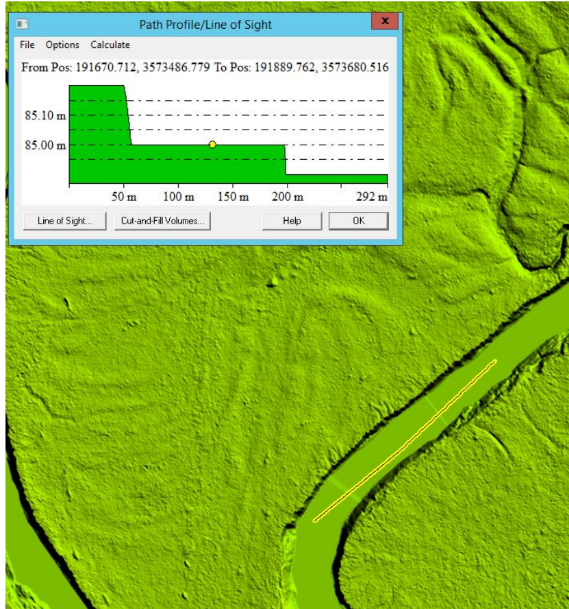
Figure 21 – Tile number 14SQA1905730. Elevation change has been stair stepped. The steps are flat from bank to bank and flow consistently downhill.
