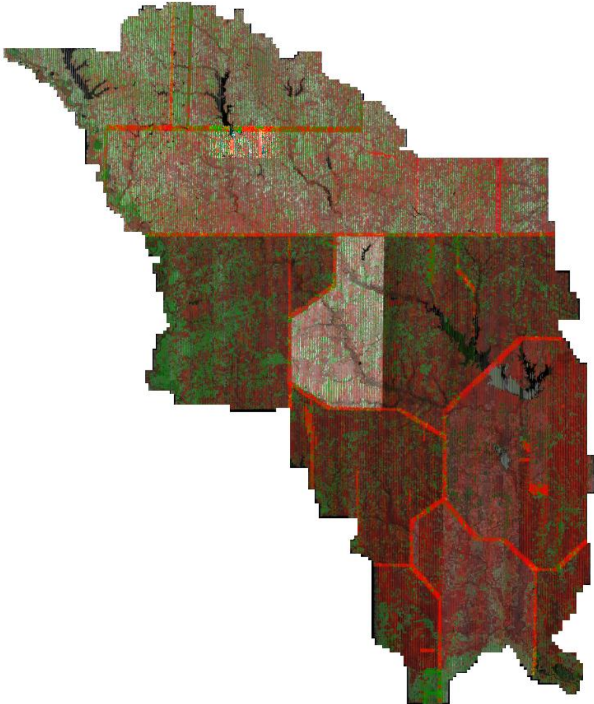
Figure 12– Single return DZ Orthos for the Texas Neches Lidar project. Inter-swath relative accuracy passes specifications.
